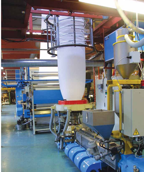
BioBag manufactures a full range of bags for food waste and yard trimmings collection, as well as makes shopping bags for retail stores. An extruder in the BioBag production facility is shown above.
