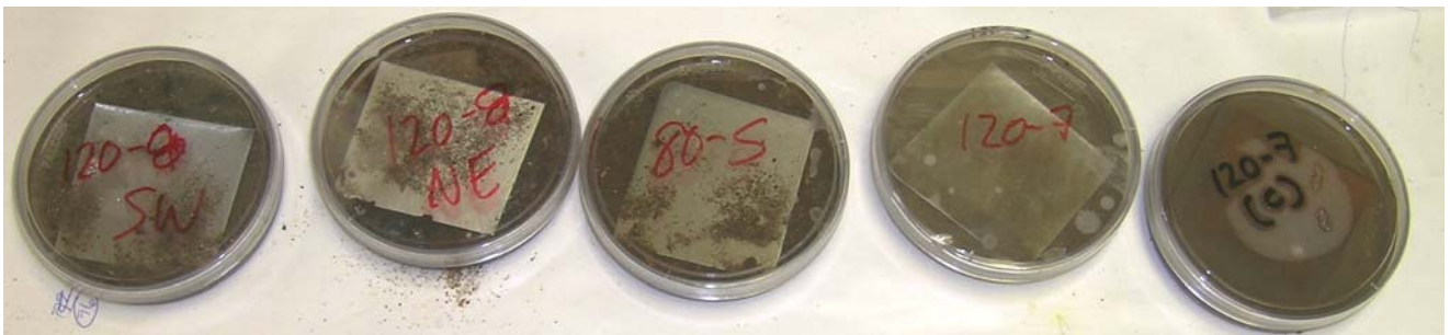
Figure 7. Corrosion test in the mixture of sand and 2% VpCI-608 solution.
