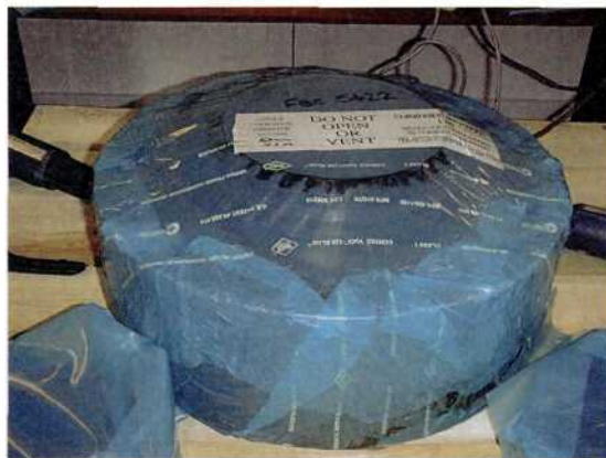
A spare flange receives protection from a thin film of inhibited grease in a VpCI polyethylene film. Photo courtesy of CSL.
