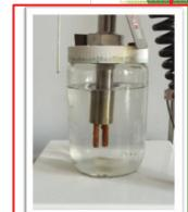
Corrosion rates in batch inhibitor application simulation, measured on LPR probe in stirred 3.5% NaCl, with stirring rod rate equal to 600 RPM.
