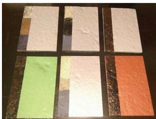
Specimens with rust converters and polymer coatings applied to surfaces prepared by different cleaning methods.
