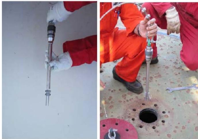
**Figure 6: Weight Loss Corrosion Coupons**
