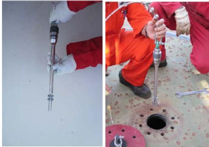
**Figure 6: Weight Loss Corrosion Coupons**
