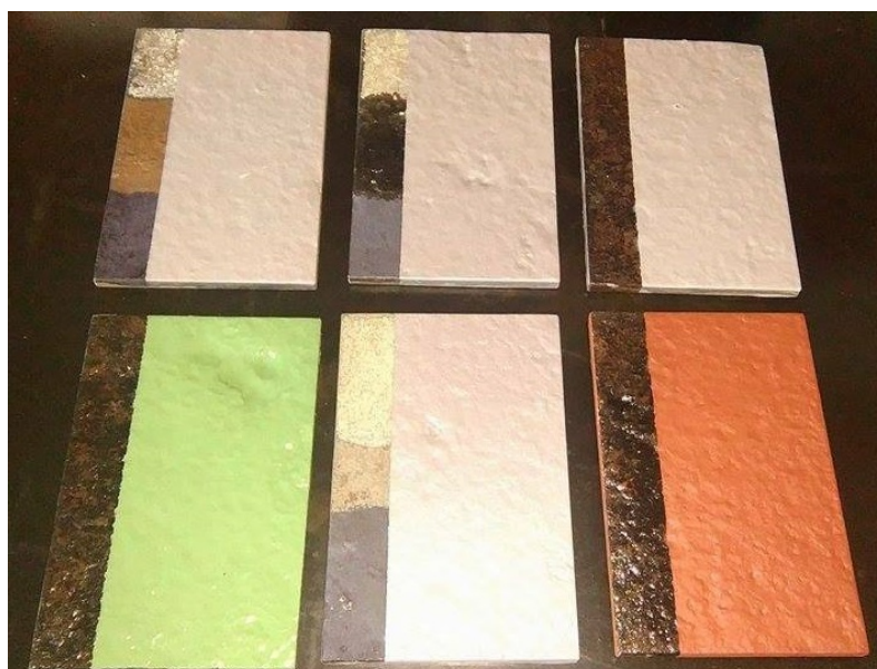
Figure 2. Specimens with applied rust converters and polymer coatings prior to EIS measurements.
