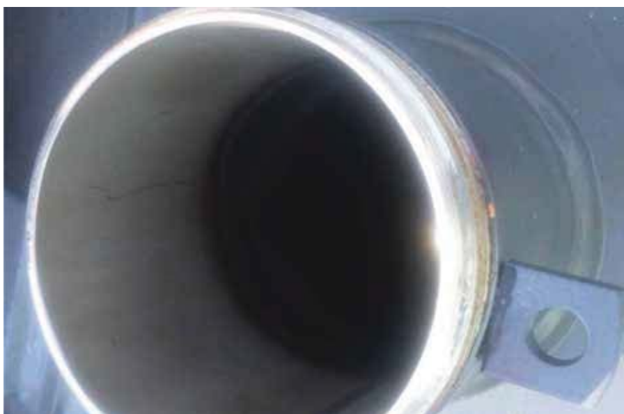
FIGURE 7 VCI-treated fuel tank after shipment. No corrosion was visible.
