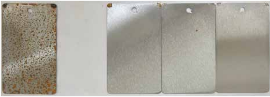
FIGURE 1. ASTM D1735 test results with Product A. The control panel is pictured on the far left.
