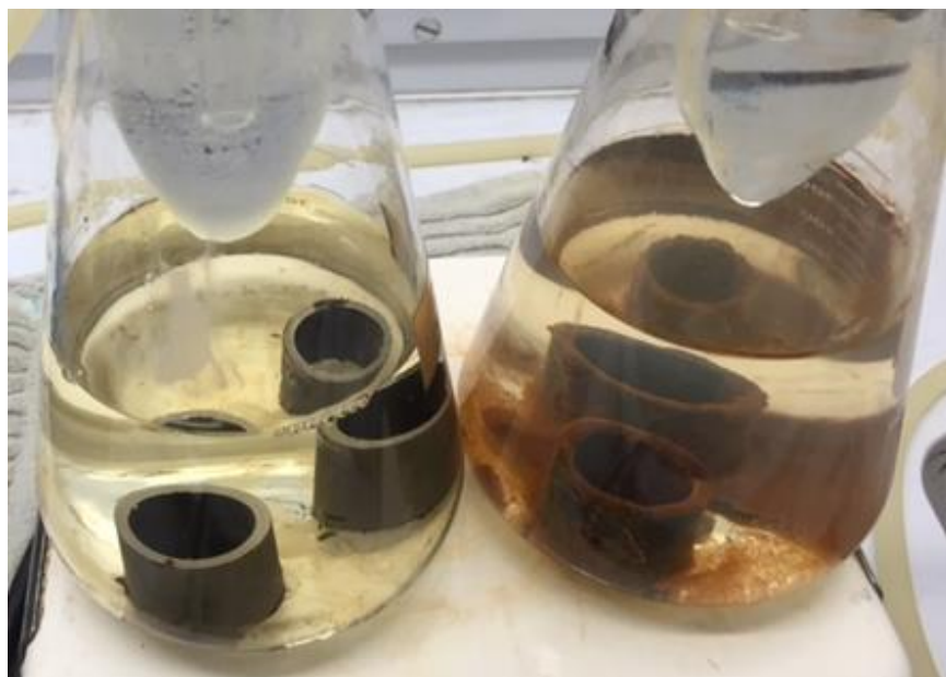
Figure 3: Corrosion test setup in boiling water solution, similar to the apparatus recommended in ASTM G123.
