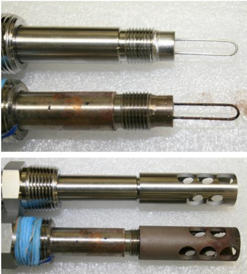
Corrosion Behavior of steel pipe in Hot Steam 90 psi, 245° F
