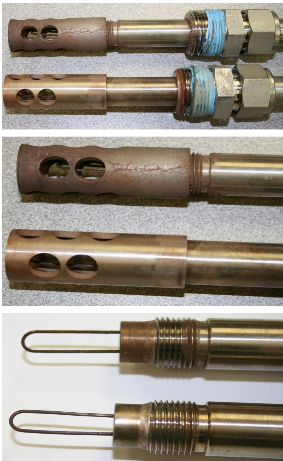
Figure 21: Comparison of corrosion ER probe surface condition of the inhibitor treated loop and control test after 2,200 hours corrosion test in hot steam/water closed loop.
