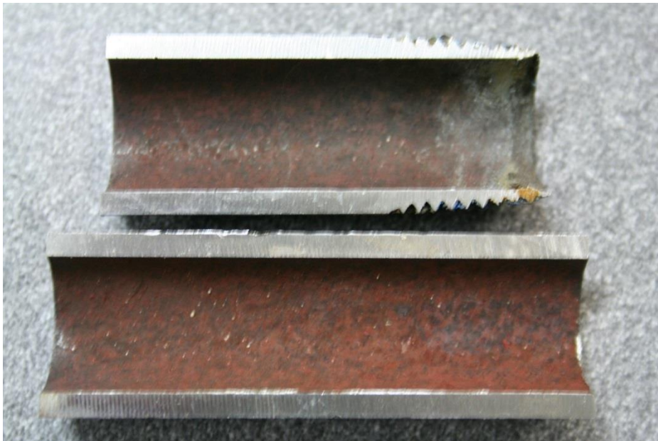
Figure 24: the steel pipe inner surface conditions of the control test after 2,100 hours corrosion test in hot steam/water closed loop.
