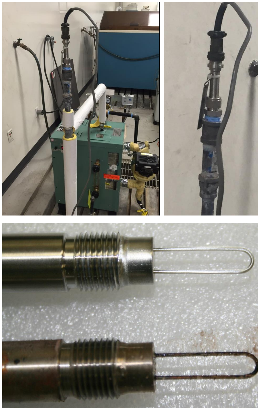
Figure 16: The Chromalox Packaged Electric Steam and hot water boiler with its closed loop piping system used for the corrosion tests in the high pressure/hot steam condition. Electrical resistance (ER) probes were used to monitor corrosion rate during testing.
