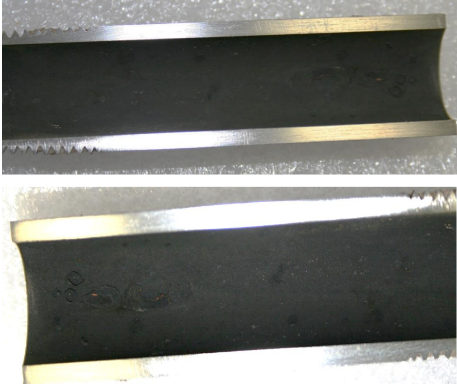
Figure 23: the steel pipe inner surface conditions of the inhibitor treated loop after 2,200 hours corrosion test in hot steam/water closed loop.
