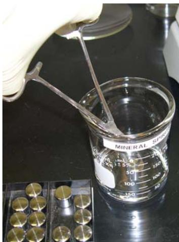
**FIGURE 6: Forceps being used to place prepared steel specimens into the cleaning beaker.<sup>(7)</sup>**
