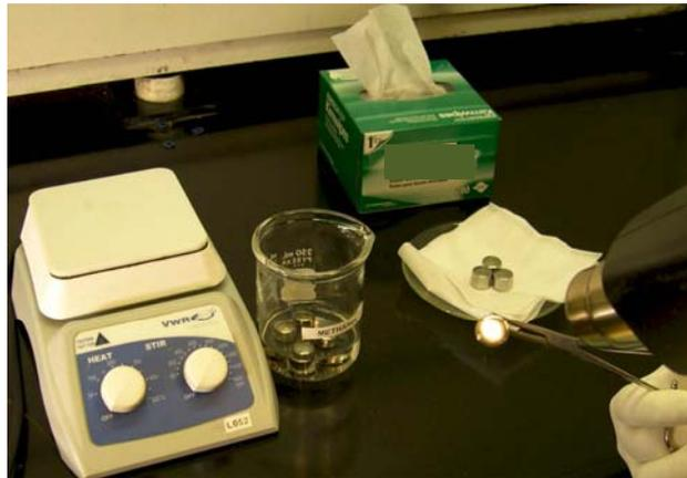
**FIGURE 8: Specimen, held with clean forceps in a gloved hand, being dried by a heat gun. Several dried specimens are temporarily held on an absorbent lint-free laboratory wipe.<sup>(9)</sup>**
