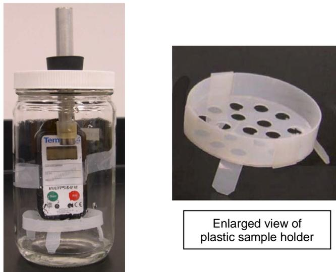
**FIGURE 4: Datalogger inside the jar-test apparatus, held in place with low-acid transparent adhesive tape.<sup>(4)</sup>**
