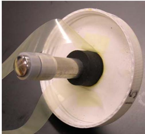
**FIGURE 9: VIA-Ferrous test jar lid (internal view) showing steel specimen inserted in the end of the silicone tubing with VCI material sample strips held in place with low-acid transparent adhesive tape.<sup>(10)</sup>**
