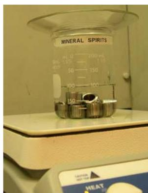
**FIGURE 7: Hot plate with cleaning beaker covered with watch glass to reduce evaporation.<sup>(8)</sup>**
