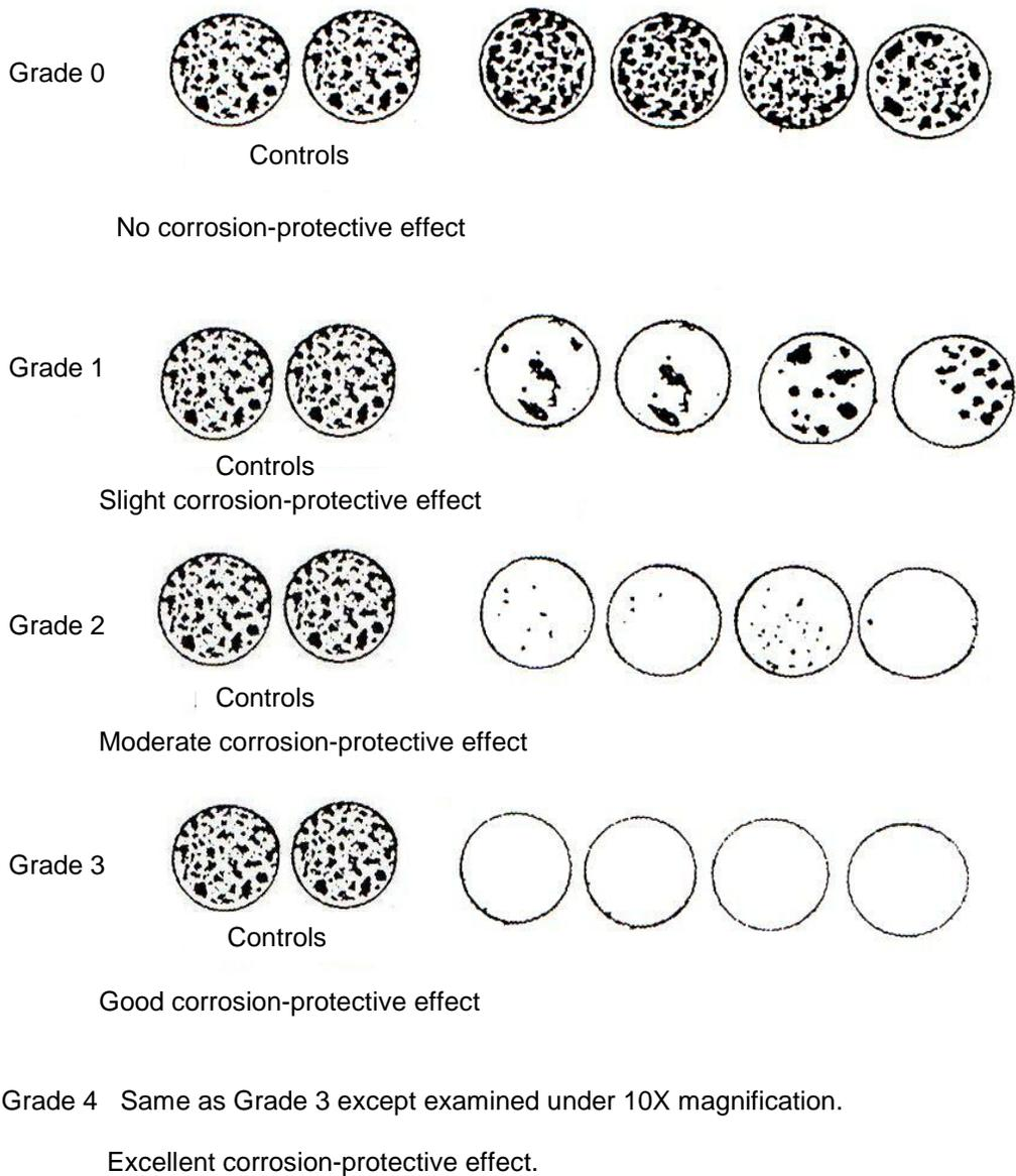
**FIGURE 12: Typical visual patterns for rating the group of specimens.<sup>(13)</sup>**
