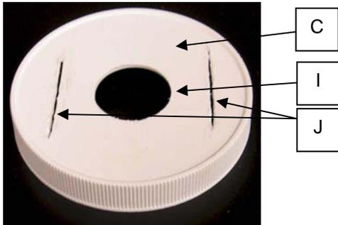
C. Lid, plastic, with screw threads to fit the standard liter (quart) size jar (Figure 1, Item D), with drilled center hole
