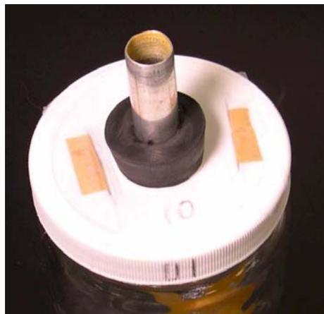
**FIGURE 10: VIA-Ferrous test jar lid (external view) showing VCI material sample strips inserted through slots in lid and held in place with low-acid transparent adhesive tape.<sup>(11)</sup>**
