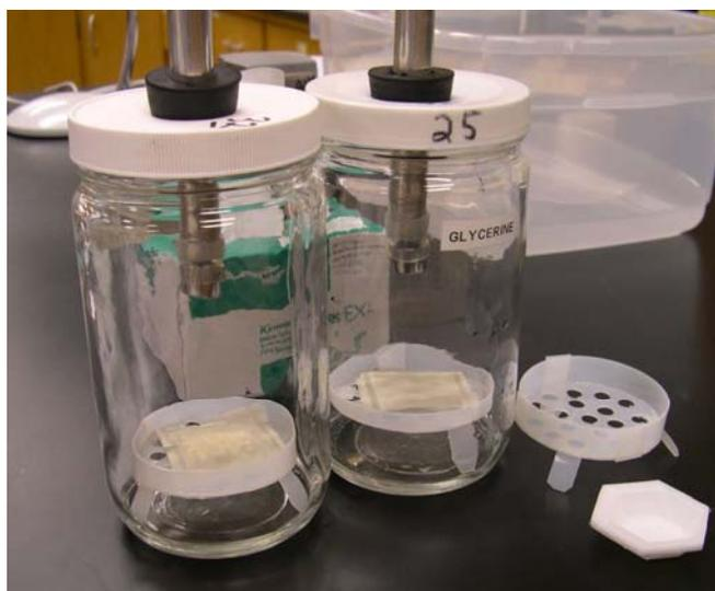
**FIGURE 11: Examples of sample holders for powder, pellet, and liquid forms of VCI materials.<sup>(12)</sup>**
