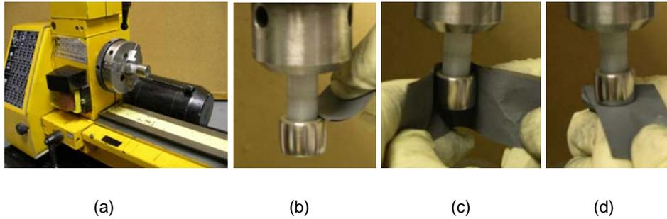
**FIGURE 5: Steel specimen on spindle in chuck of a horizontal lathe (a) and in chuck of a vertical drill press being polished on the top (b), side (c), and bottom (d) with abrasive paper.<sup>(6)</sup>**
