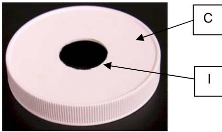
C. Lid, plastic, with screw threads to fit the standard liter (quart) size jar (Figure 1, Item D), with drilled center hole
