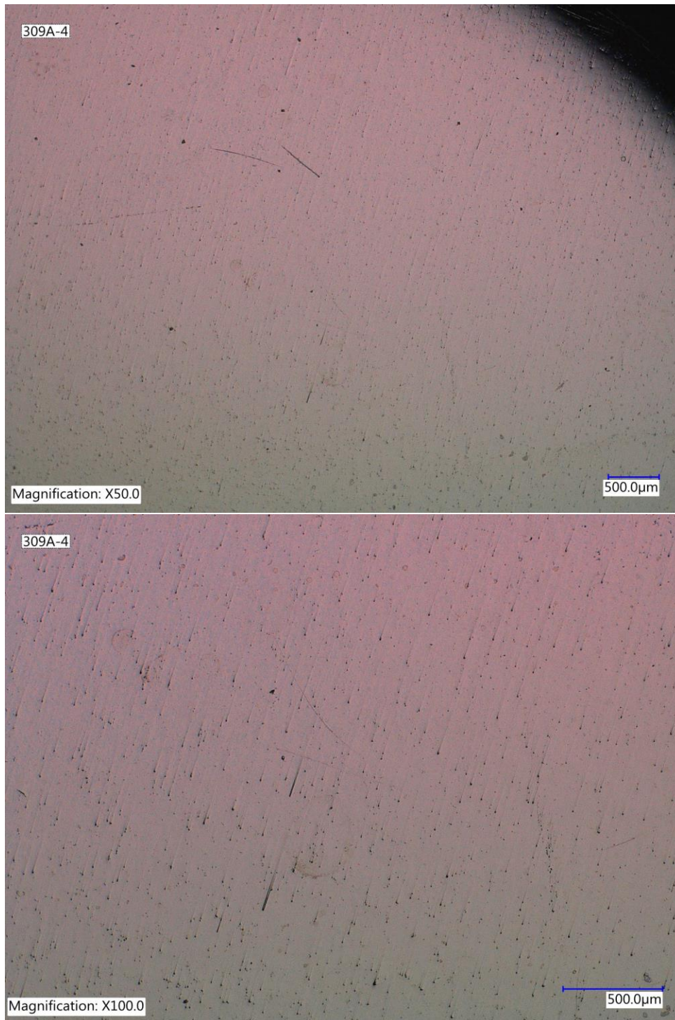
Fig. 8: Optical micrographs of the sample #4 exposed VpCI 309A in TM0208 VIA test, Grade 3.
