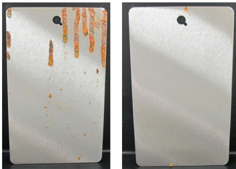
Figure 1: Panels at end of Accelerated Corrosion test Control (left), Sample with VCI-2 (right)
