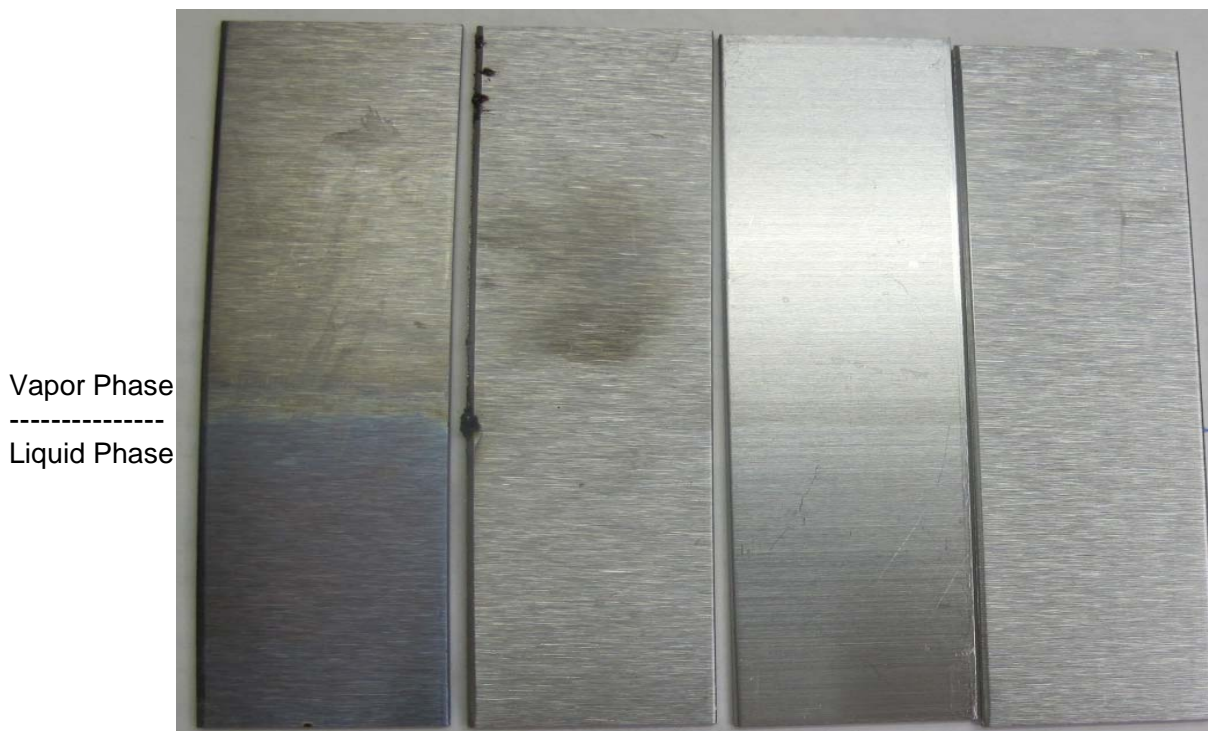
Salt of A Salt of C Salt of B Petro VCI Figure 3: Partial Immersion in Solution of Ammonium Salt of Aromatic Acids In Tap Water (10months)
