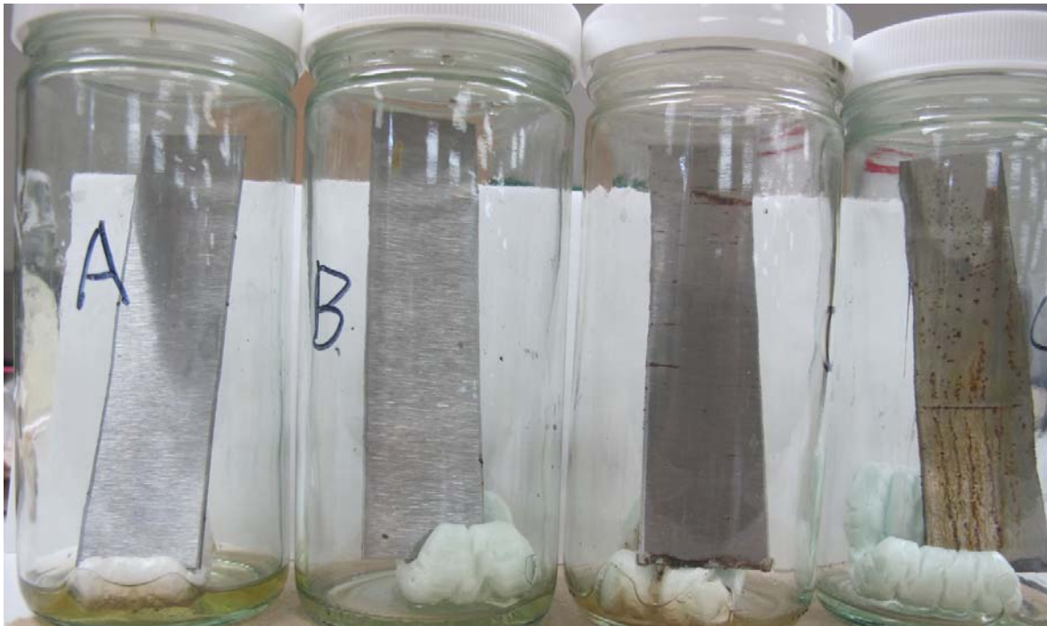
Figure 2: Setup of Corrosion Testing in Hydro Testing
