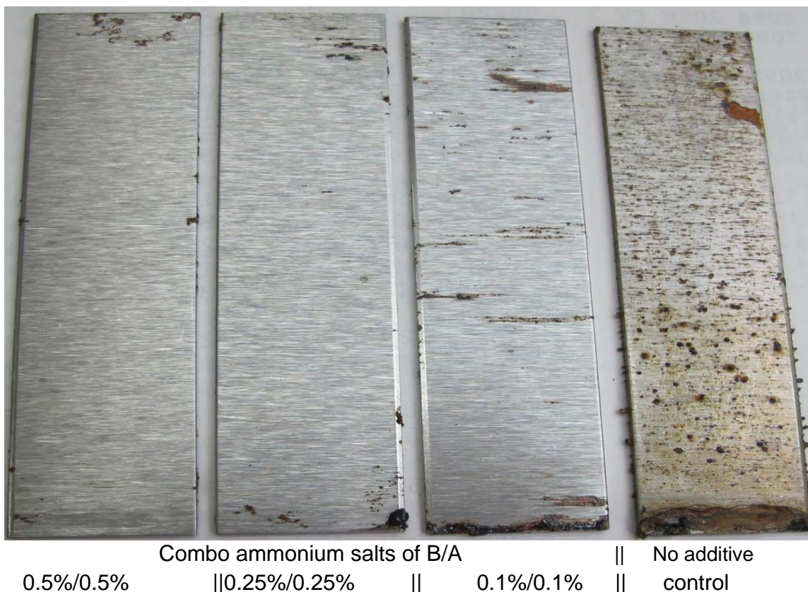
Figure 4: 7 Days after Salty Hydro Testing Fluid Was Drained
