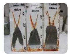
**FIGURE 7.** Control sample, 540 h of continuous salt spray.
