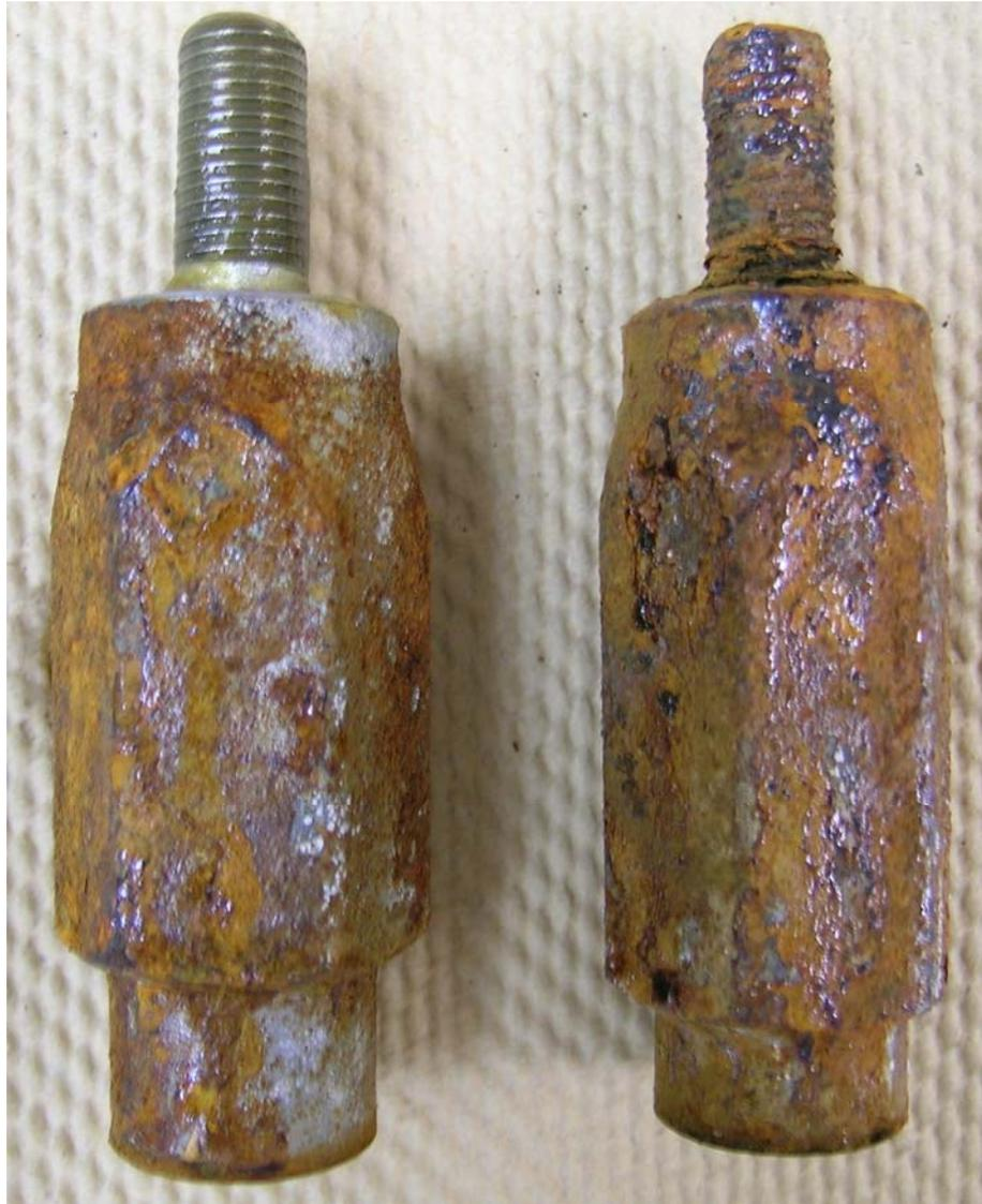
366 hours in ASTM B 117 Salt Spray Cabinet. VpCI-369 on left, Black Oxide coating on the right.
