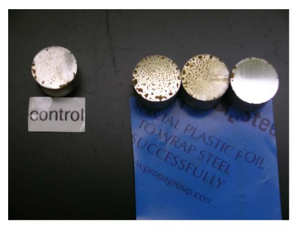
**Conclusion:** The submitted film failed both Razor Blade Test and VIA Test, which means that it doesn't protect steel either in vapor or in contact phases.
