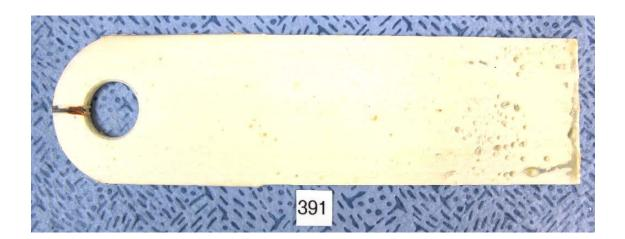
**Interpretations:** Of the four products tested, EcoLine 3690 provided the best corrosion protection in ASTM D-1748 humidity cabinet conditions. The remaining three products also provided excellent protection.
