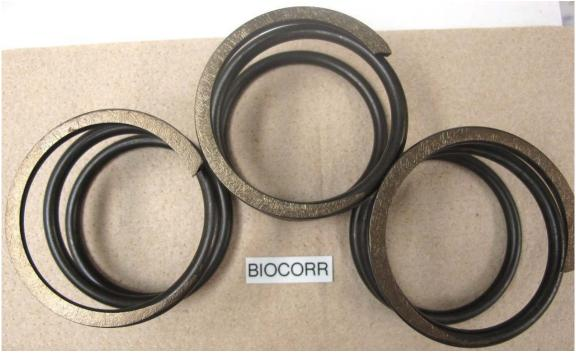
**Interpretations:** After over 900 hours in accelerated corrosion testing, BioCorr
