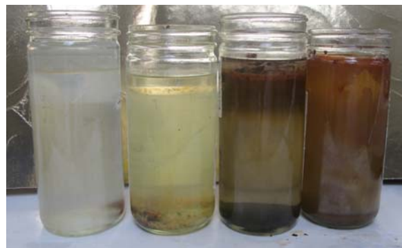
Picture 2: Aligned from left to right are MCI-2018, Protectosil CIT, Protectosil 300, and the control.
