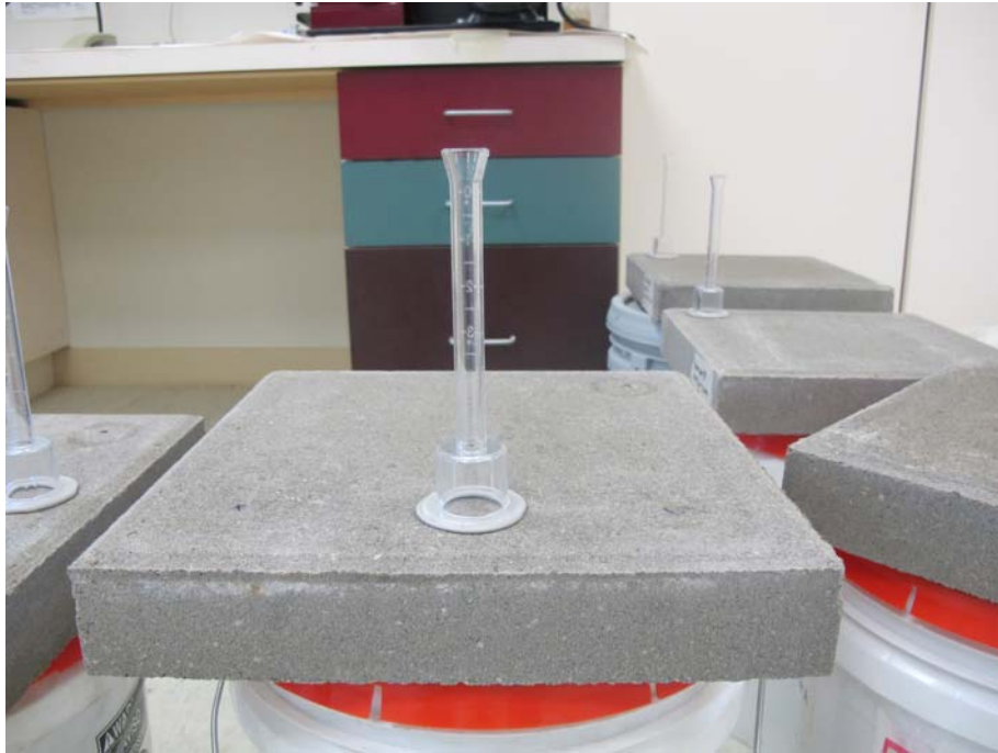
Picture 1: Rilem tube attached to the surface of a masonry block
