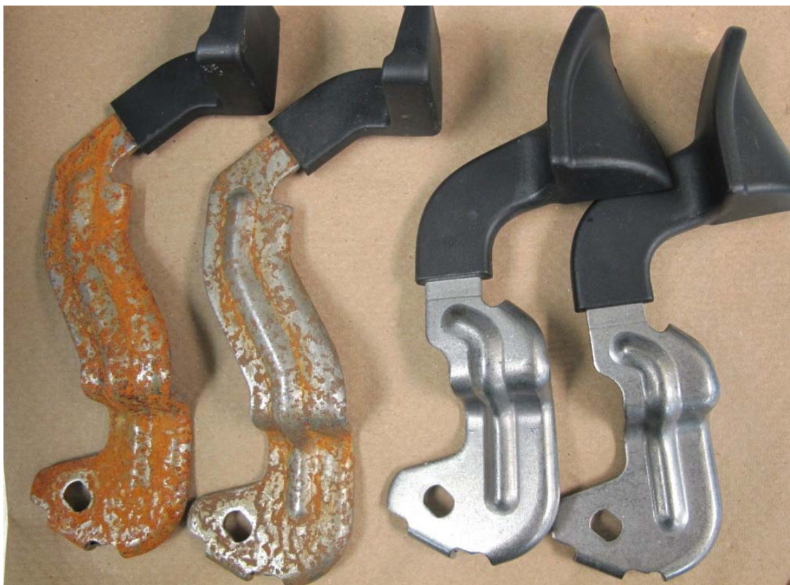
Figure 2: Group B parts after 696 hours of ASTM D-1735 testing. From L-R: Current RP only, BioCorr only, Current RP/Armor, VpCI-126/BioCorr
