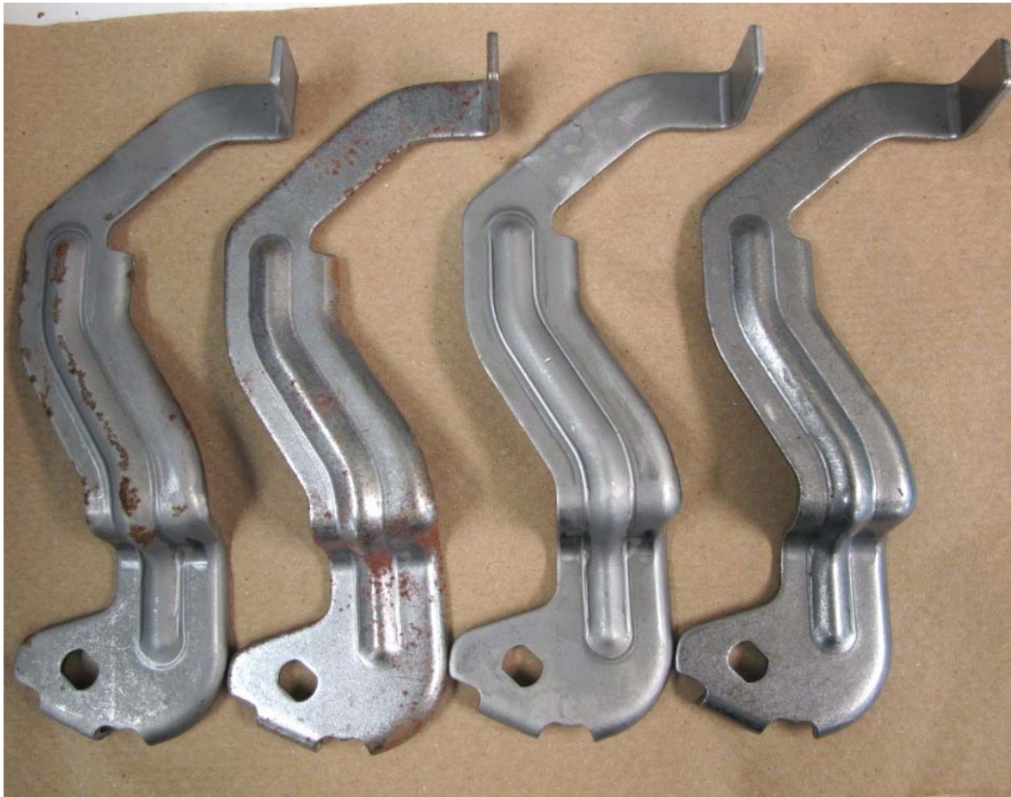
Figure 1: Group A parts, after 696 hours of ASTM D-1735 testing. From L-R: Amor/Current RP, Armor/BioCorr, VpCI-126/Current RP, VpCI-126/BioCorr
