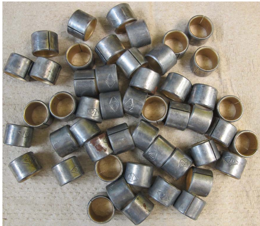
Figure 3: VpCI-416/126 treated parts, after 336 hours of testing.
