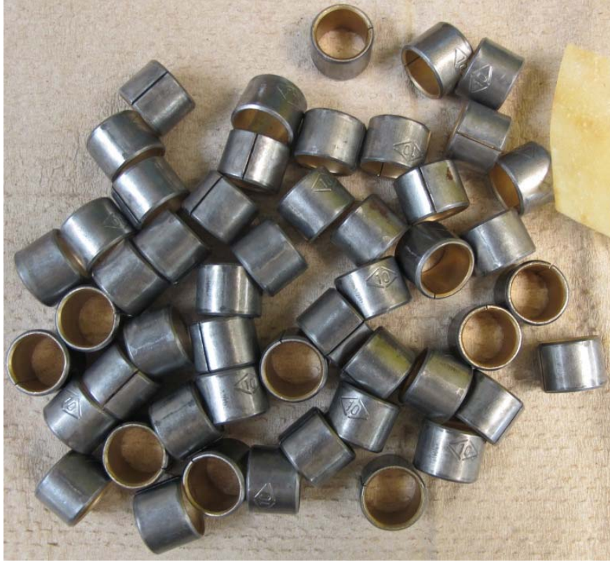
Figure 4: VpCI-416/126/BioPad treated parts, after 336 hours of testing.
