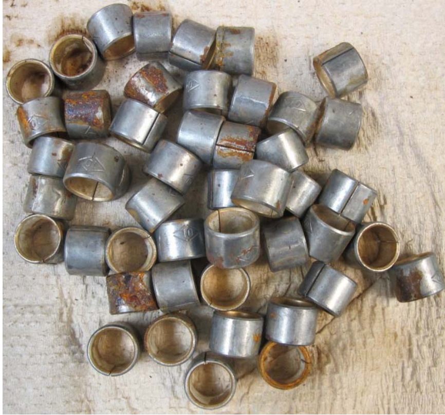
Figure 2: Dry Coat/Armor VCI treated parts, after 336 hours of testing.
