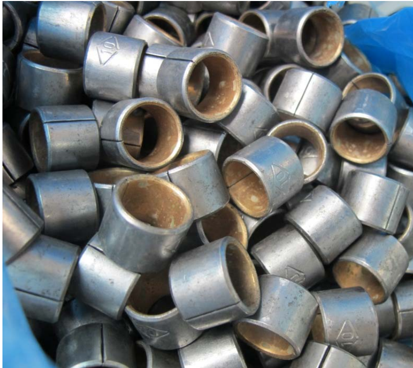
Figure 1: Bushings found to be corroded upon receipt. These parts were not tested.
