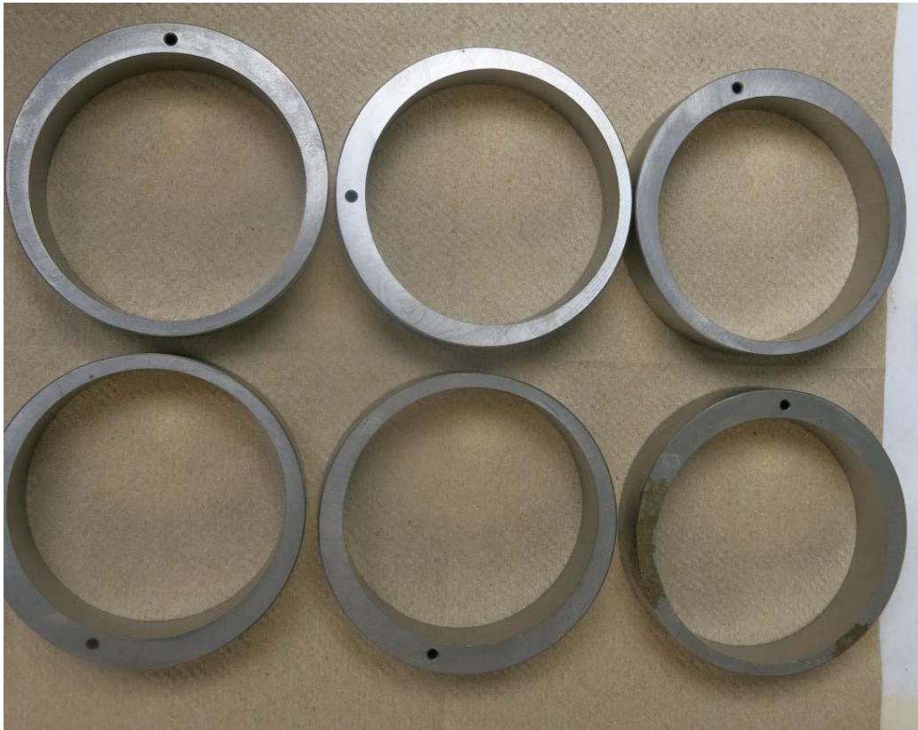
Figure 2: VpCI-126 packed parts, after 432 hours in ASTM D-1735 testing.
