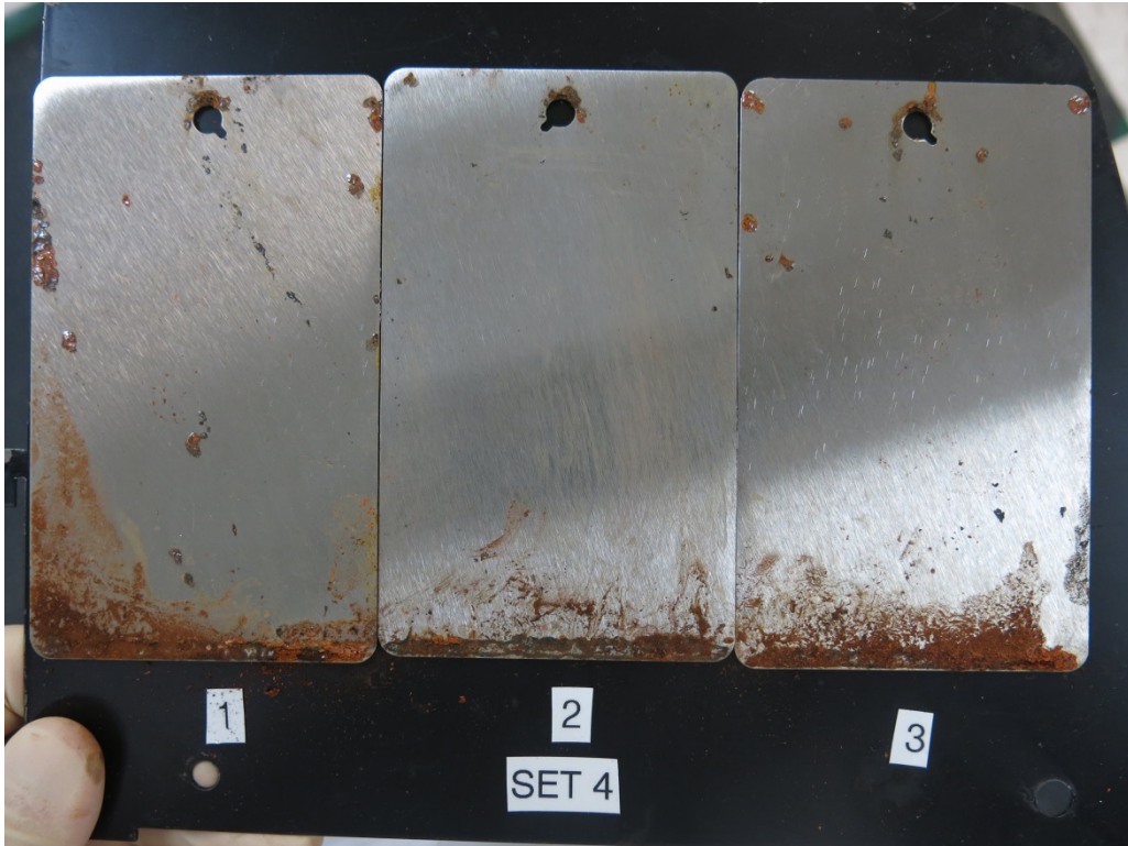
Picture 5: The Synlube and Techniclean-treated panels after 500 hours in the humidity cabinet
