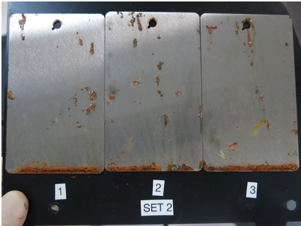
Picture 3: The Techniclean-treated panels after 500 hours in the humidity cabinet
