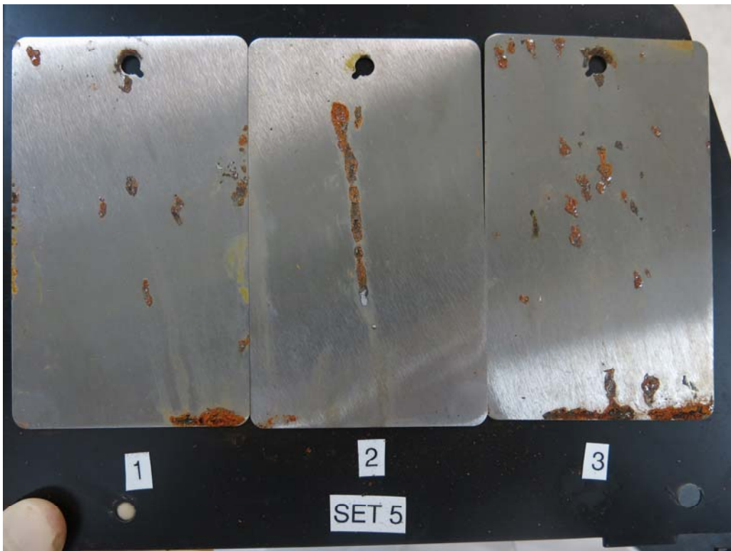
Picture 6: The coolant-treated panels after 500 hours in the humidity cabinet
