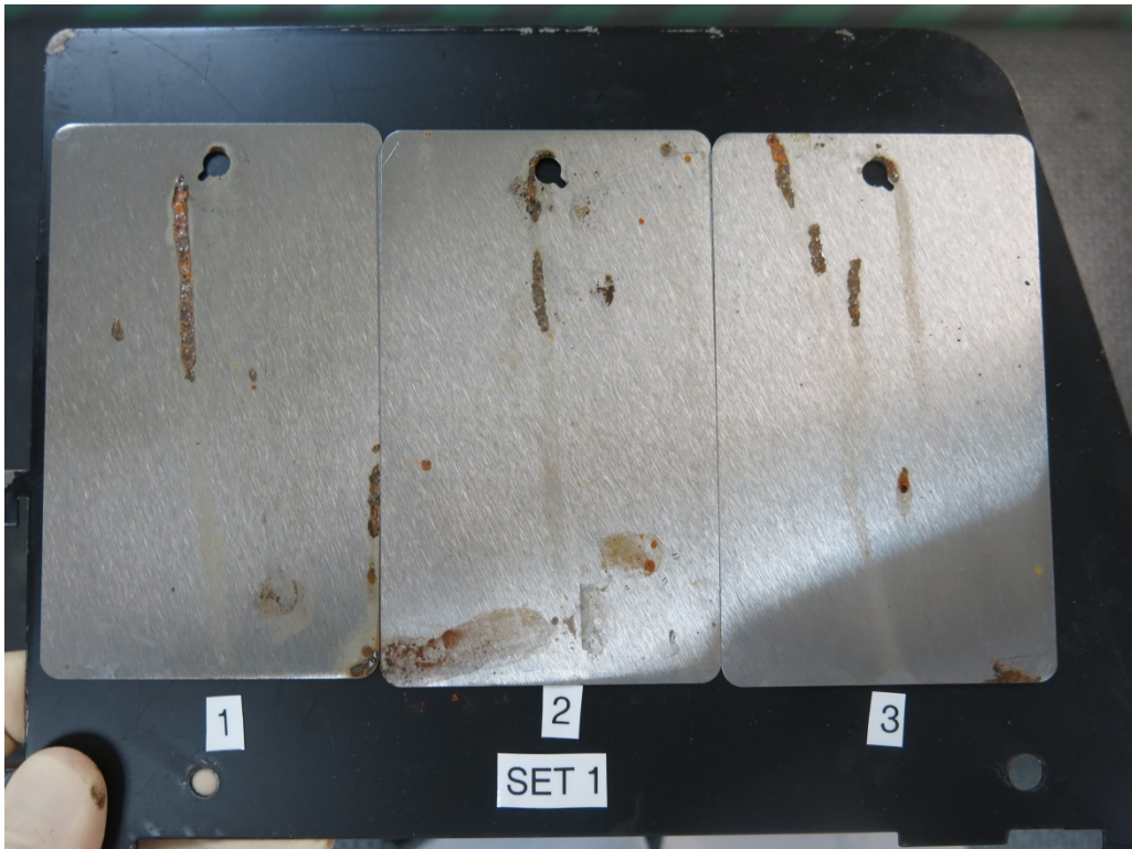
Picture 2: The Rustillo-treated panels after 500 hours in the humidity cabinet
