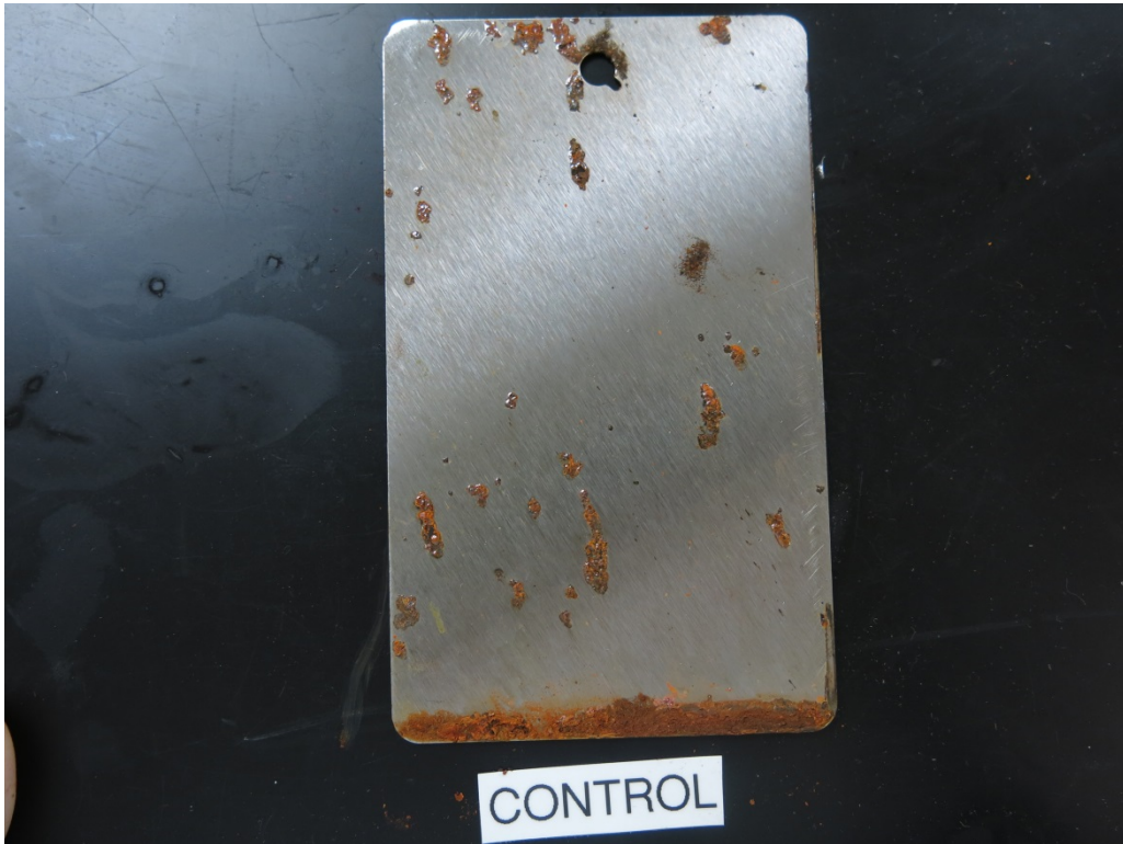
Picture 1: The untreated control panel after 500 hours in the humidity cabinet
