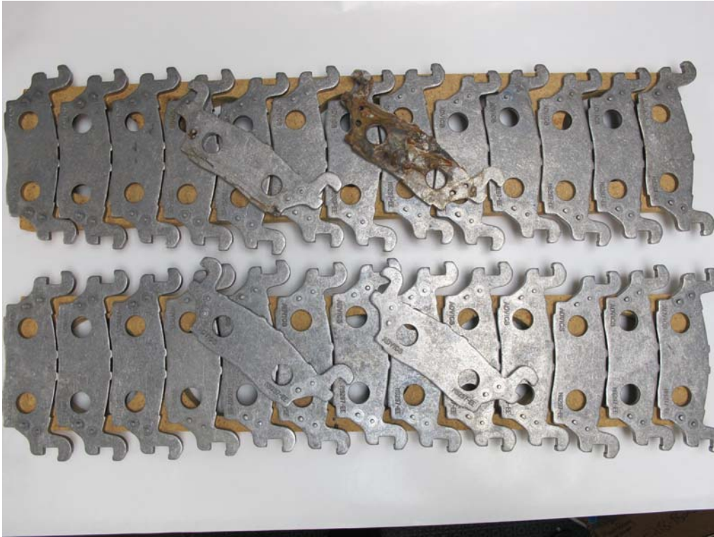
Picture 1: An overview of all parts from both bags after 360 hours in the humidity chamber. The top row is from the Armor-protected bag while the bottom row is from the Cortec-protected bag.
