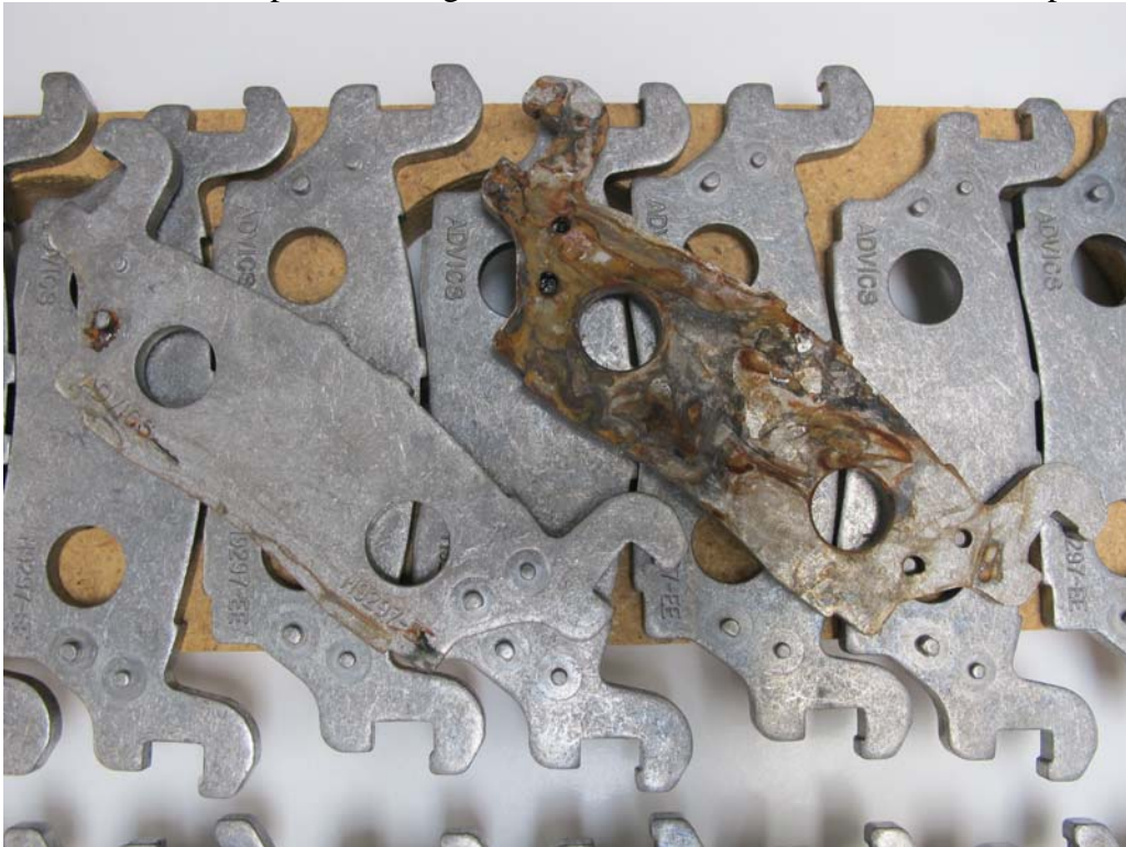
Picture 2: A closer image of the Armor-protected parts after 360 hours in the chamber. These were the parts in the bottom of the bag.
