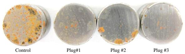
Cortec's VpCI-126 film (tested with two 1"x6" strips of film per jar)
