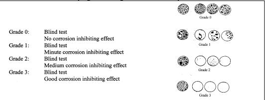
**Interpretations:** The three submitted films do not provide sufficient contact or vapor phase corrosion protection, based on results of VIA and razor blade testing.
