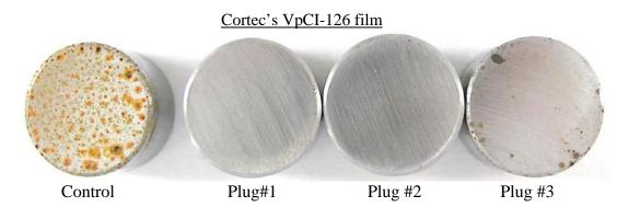
VIA Test Grades (Grade 2 or 3 are passing) All three plugs must be grade 2 or better to pass the test
