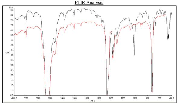
Above: Caliburn film (Black, higher %T) compared to control PE (Red, lower %T)
