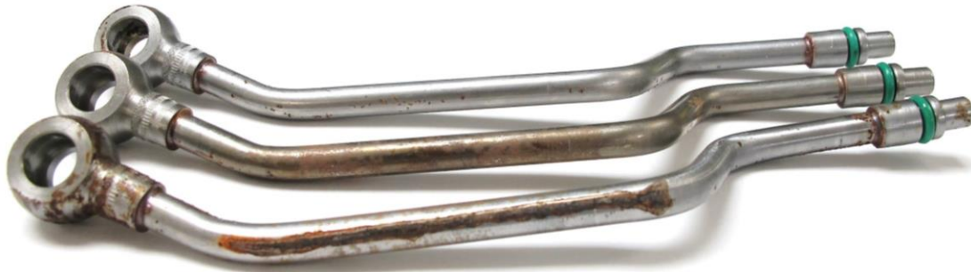
Control parts sealed in plain polyethylene film
