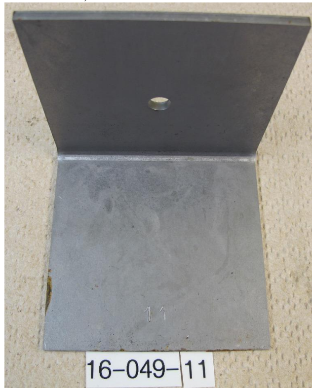
Figure 12: Part 11, after 522 hours in ASTM D-1735 testing.
