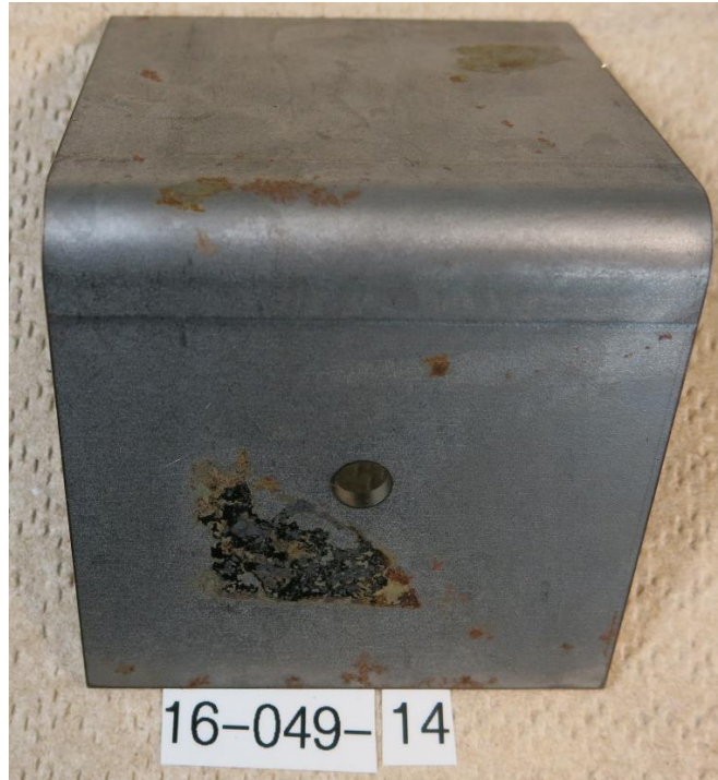
Figure 16: Part 14 (opposite side), after 522 hours of ASTM D-1735 testing.
