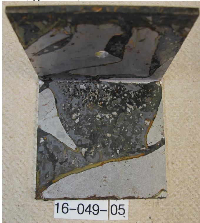
Figure 6: Part 5, after 522 hours in ASTM D-1735 testing.
