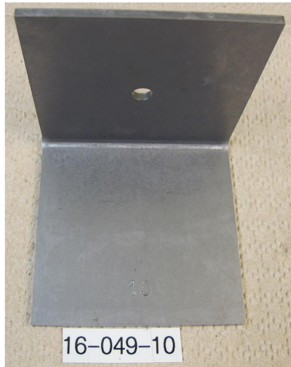
Figure 11: Part 10, after 522 hours in ASTM D-1735 testing.
