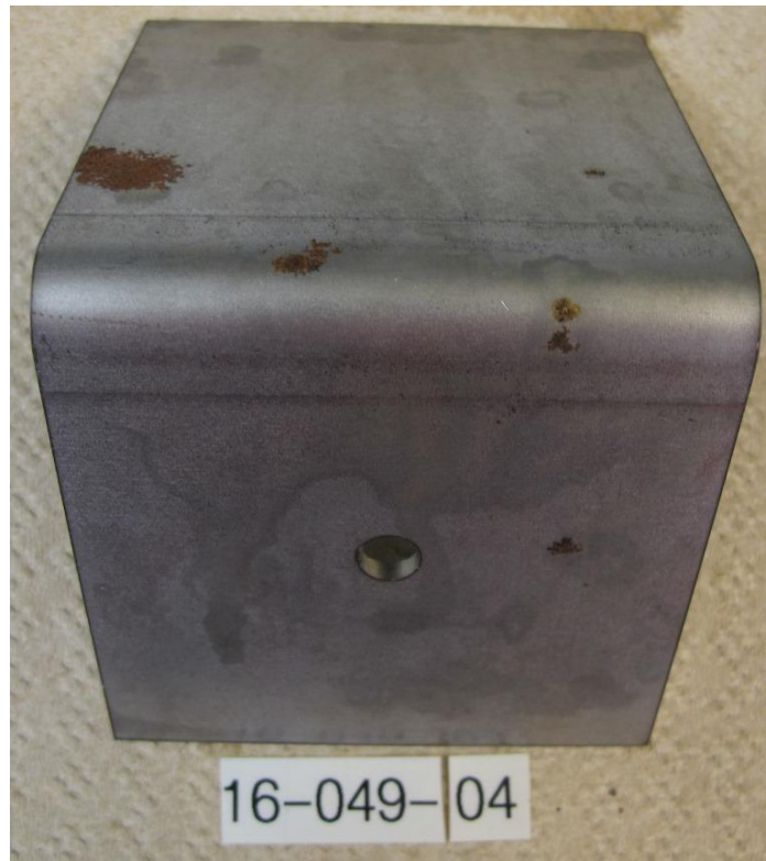
Figure 5: Part 4 (opposite side), after 522 hours in ASTM D-1735 testing.
