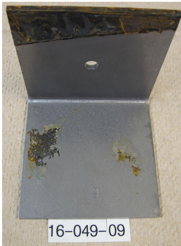
Figure 10: Part 9, after 522 hours in ASTM D-1735 testing.
