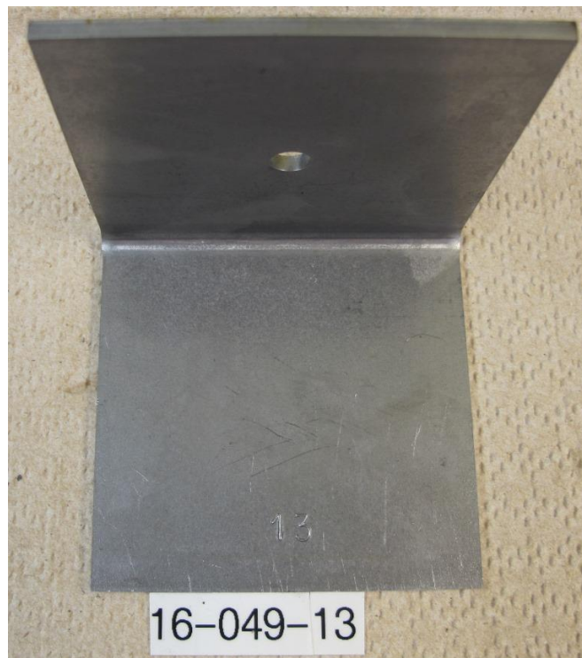
Figure 14: Part 13, after 522 hours in ASTM D-1735 testing.
