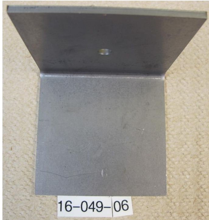
Figure 7: Part 6, after 522 hours in ASTM D-1735 testing.
