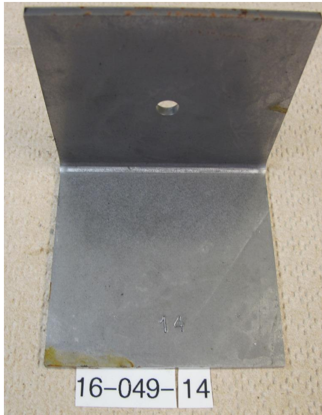
Figure 15: Part 14, after 522 hours in ASTM D-1735 testing.
