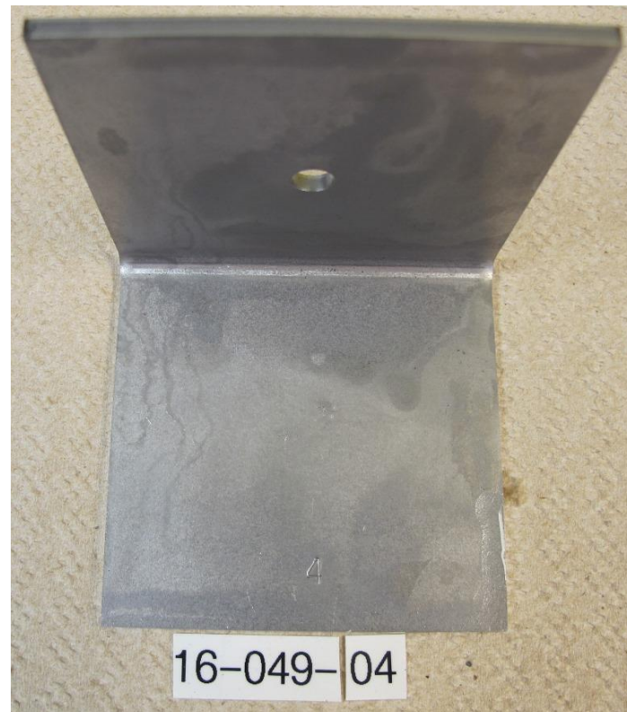
Figure 4: Part 4, after 522 hours in ASTM D-1735 testing.
