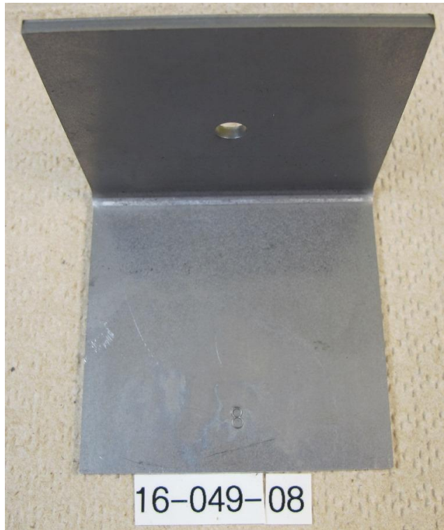
Figure 9: Part 8, after 522 hours in ASTM D-1735 testing.
