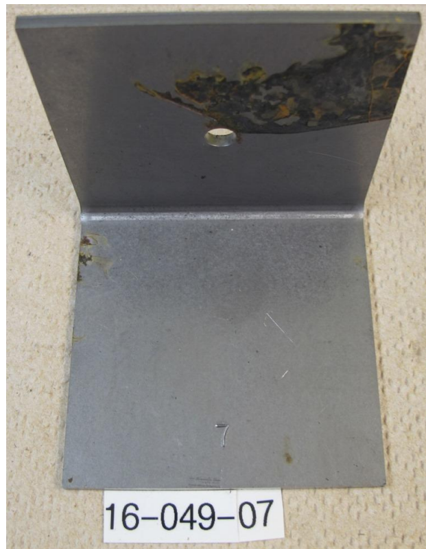
Figure 8: Part 7, after 522 hours in ASTM D-1735 testing.
