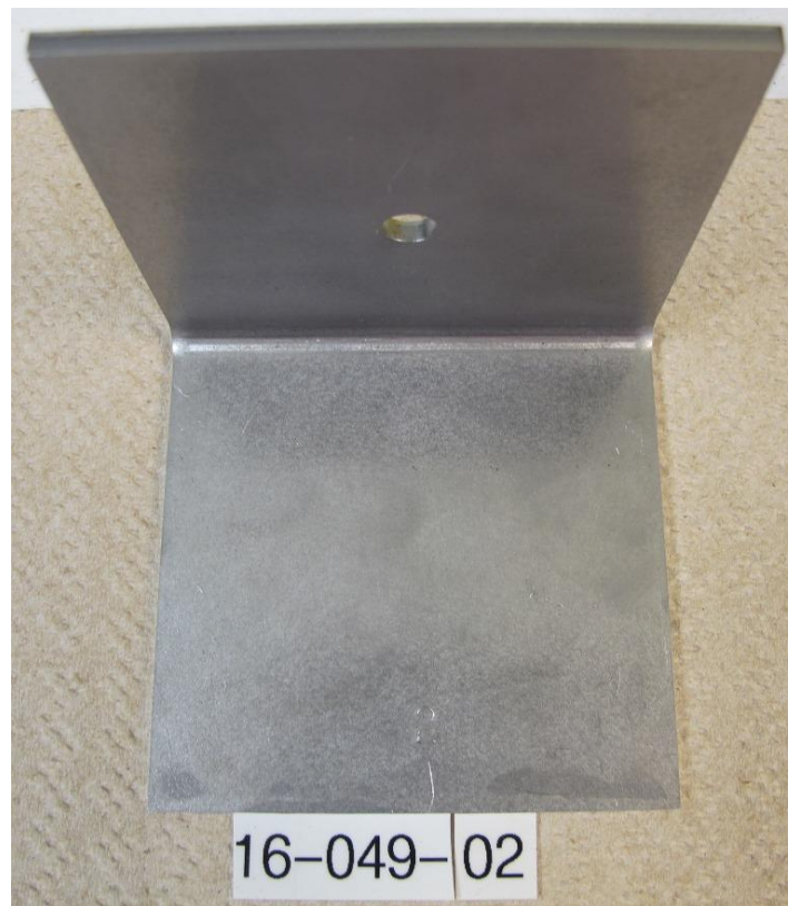
Figure 1: Part #1, after 522 hours in ASTM D-1735 testing.
