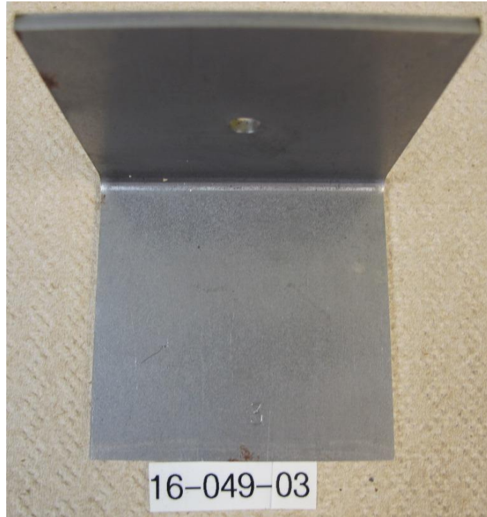
Figure 3: Part #3, after 522 hours in ASTM D-1735 testing.
