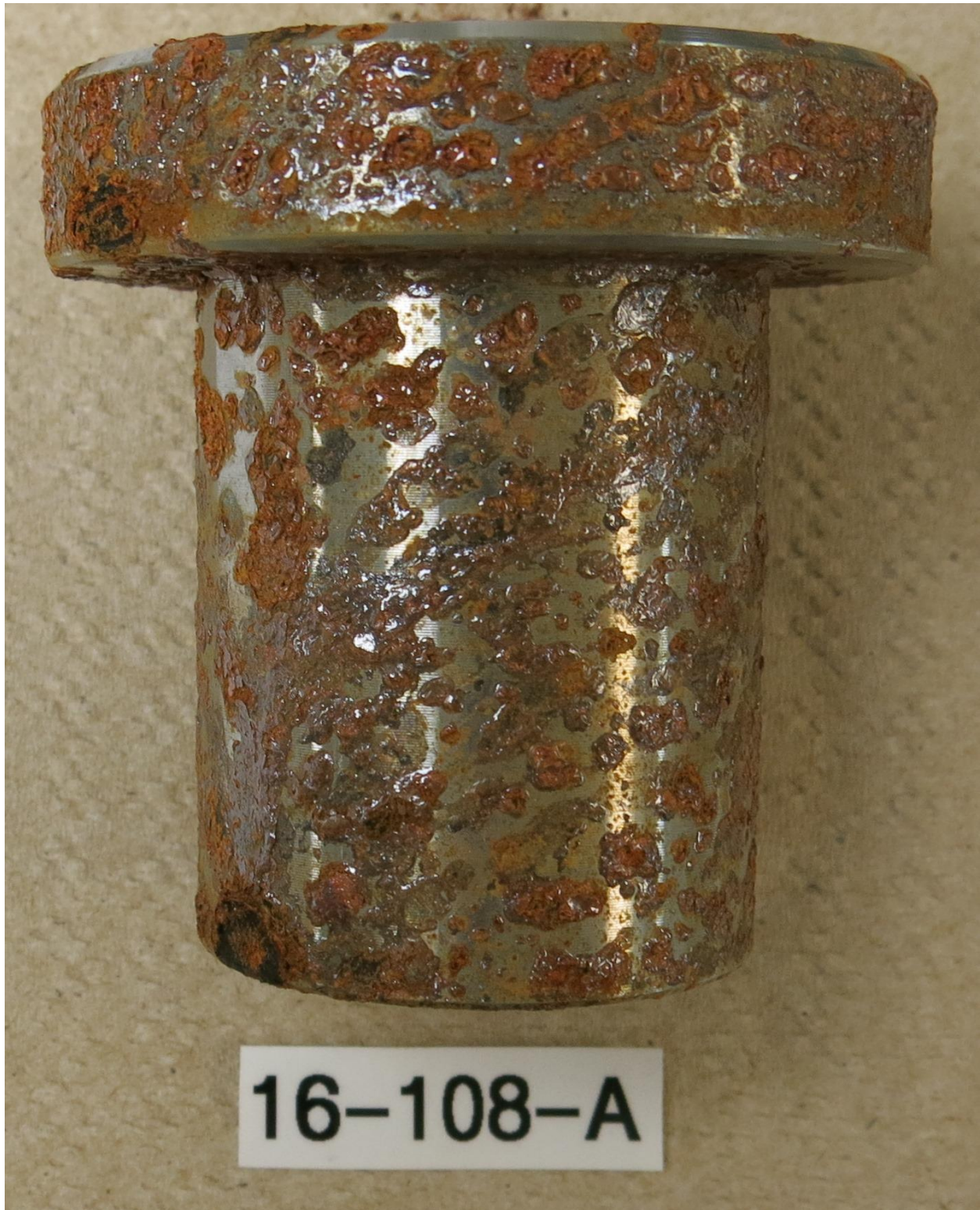
Figure 1: Part 16-108-A (control), after 336 hours in ASTM D1748 testing.
