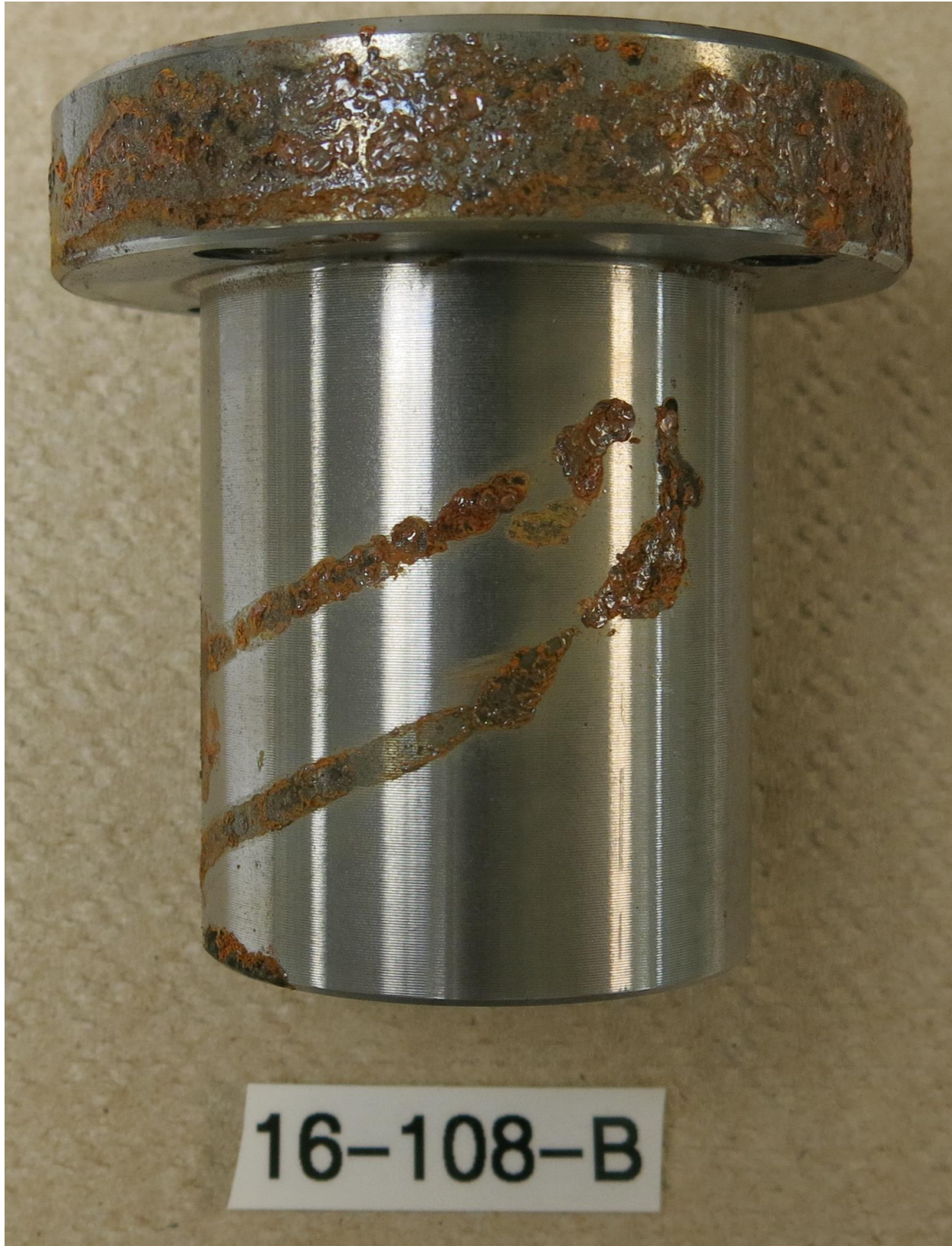
Figure 2: Part 16-108-B, treated with Rilco RP-184, after 336 hours in ASTM D-1748 testing.
