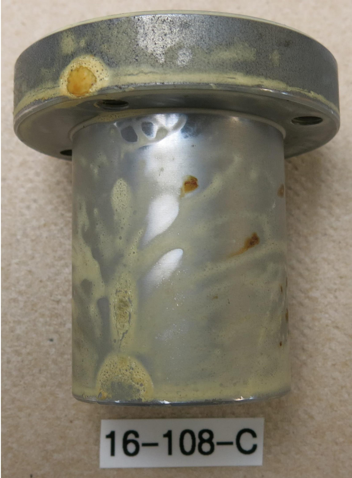
Figure 3: Part 16-108-C, treated with VpCI-389D, after 336 hours in ASTM D-1748 testing.
