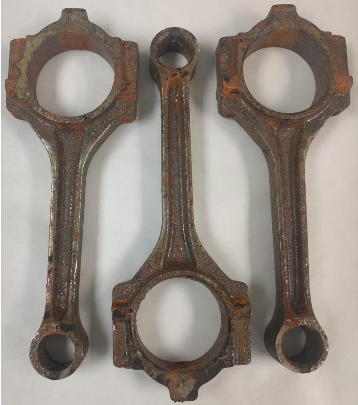
Photo 1: Control connecting rods, after 744 hours in accelerated corrosion testing.
