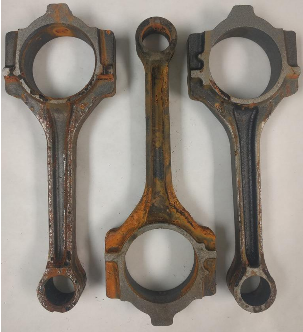
Photo 2: Protexo 1125 treated connecting rods, after 744 hours in accelerated corrosion testing.
