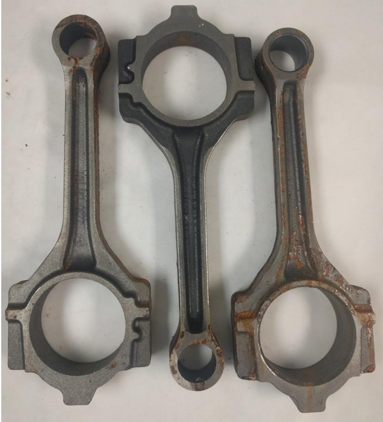
Photo 3: VpCI-325 treated connecting rods, after 744 hours in accelerated corrosion testing.
