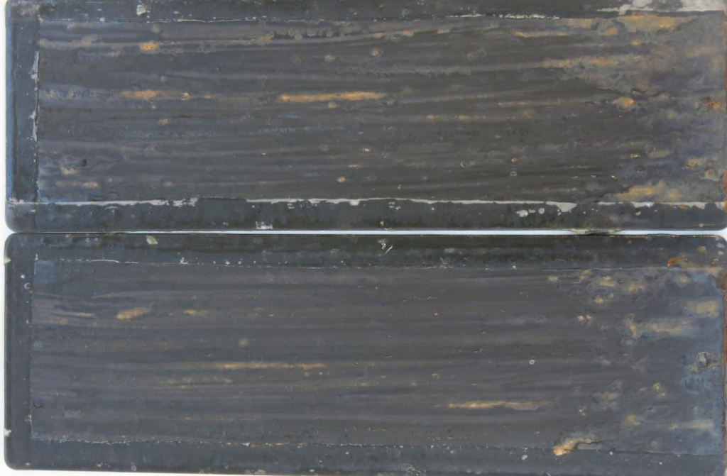
Figure 6: Corro Seal panels after 360 hours in salt spray chamber (4.7-5.0 mil DFT)
