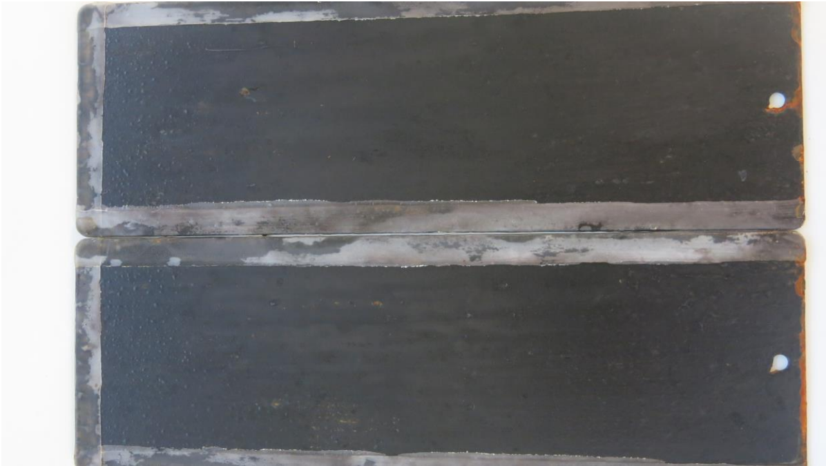
Figure 4: CorrVerter panels after 360 hours in salt spray chamber (2.1-2.4 mil DFT)
