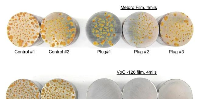
VIA Test Grades (Grade 2 or 3 are passing) All three plugs must be grade 2 or better to pass the test Grade 0
