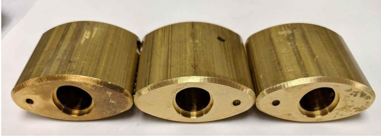
Figure 1. Padlocks after 596 hours using current method (1). Cleaned with EverCycle 411, followed by two water rinses. Significant to moderate corrosion can be seen on the bottom of the padlocks.
