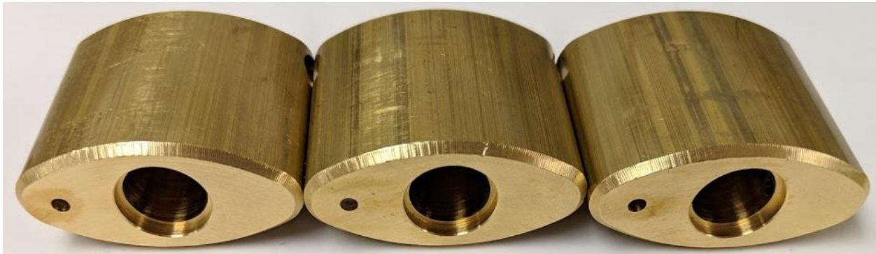
Figure 2. Padlocks after 596 hours using VpCI-418LM, VpCI-316. (Treatment method 4). Minor staining can be seen occurring on the bottom edges of the padlocks, but staining can be wiped away with a lint free wipe.
