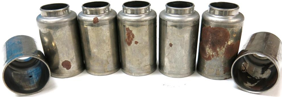
Packaged in VpCI-126 Film with one 3" x 3" Piece of BioPad (Bag #1) (showing only the corroded parts, 7 out of 54)
