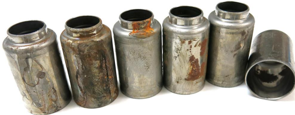
Packaged in VpCI-126 Film with one 3" x 3" Piece of BioPad (Bag #2) (showing only the corroded parts, 6 out of 54)
