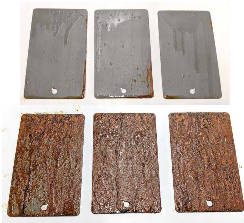
Figure 2: The panels treated with VpCI-340 CLP (top) and FrogLube CLP (bottom) after 48 hours in ASTM B117 salt spray conditions.
