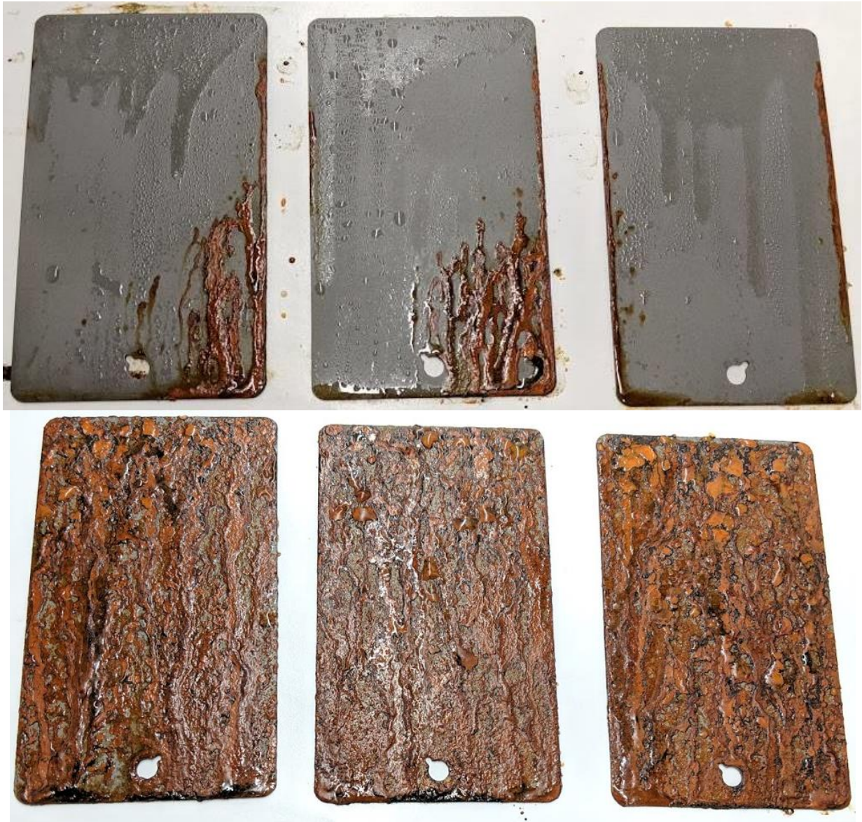
Figure 3: The panels treated with VpCI-340 CLP (top) and FrogLube CLP (bottom) after 72 hours in ASTM B117 salt spray conditions.
