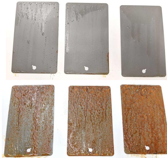
Figure 1: The panels treated with VpCI-340 CLP (top) and FrogLube CLP (bottom) after 26 hours in ASTM B117 salt spray conditions.
