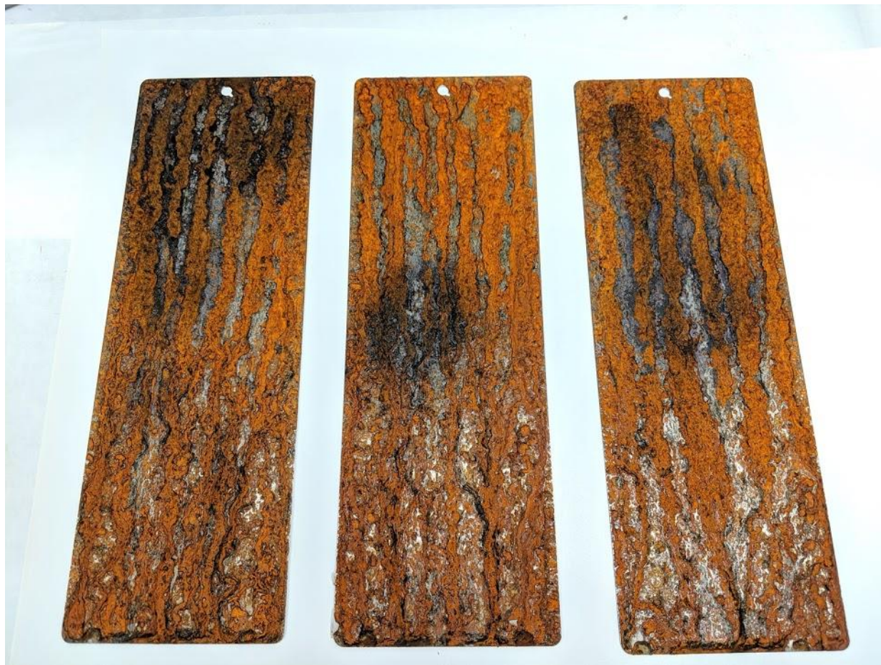
Figure 2: Panels sprayed with Total Solutions Rust Converter. Black spots appeared on the panels where the product was able to be applied, showing some degree of performance. Due to difficulty spraying the product, this test did not proceed further than pictured above.
