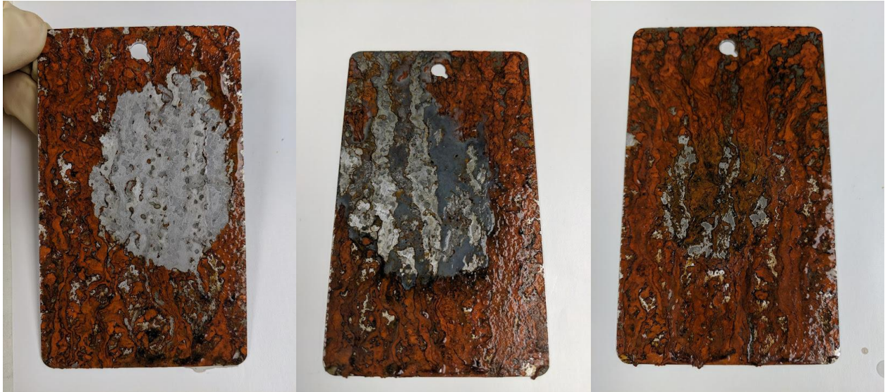
Figure 1.A: Rust remover comparison at 15 minutes. From left to right, VpCI-423, Evapo-Rust Gel, Nox-Rust Premium Rust Remover.
