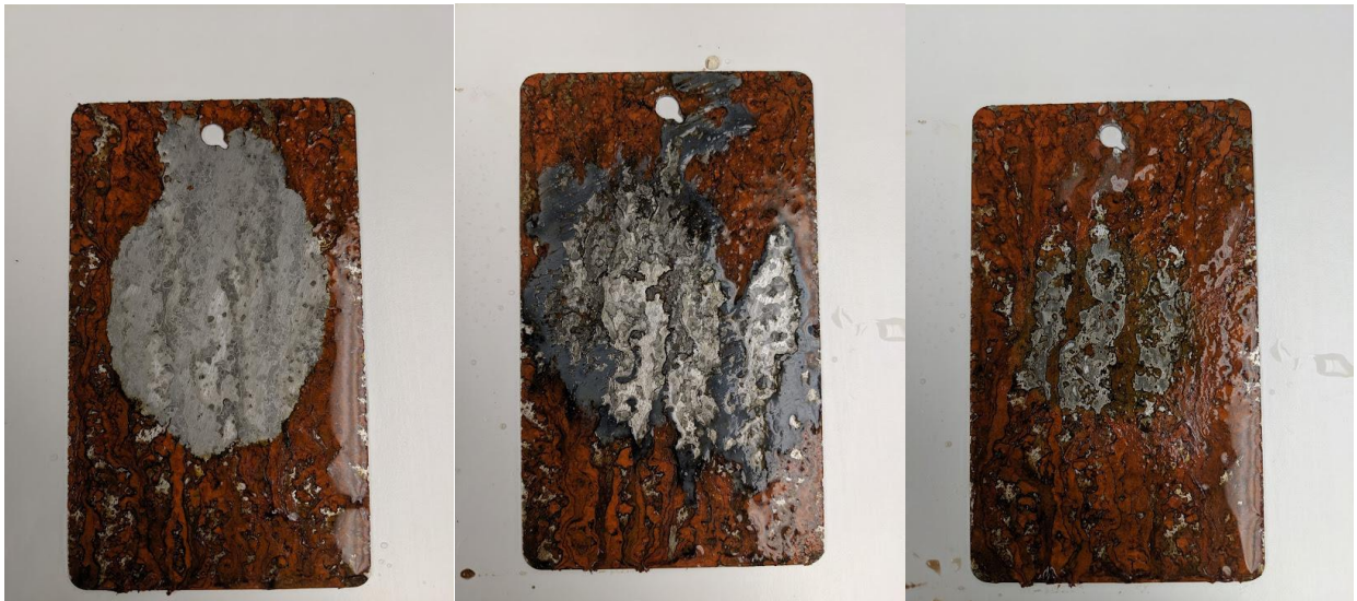
Figure 2. A: Rust remover comparison at 30 minutes. From left to right, VpCI-423, Evapo-Rust Gel, Nox-Rust Premium Rust Remover.
