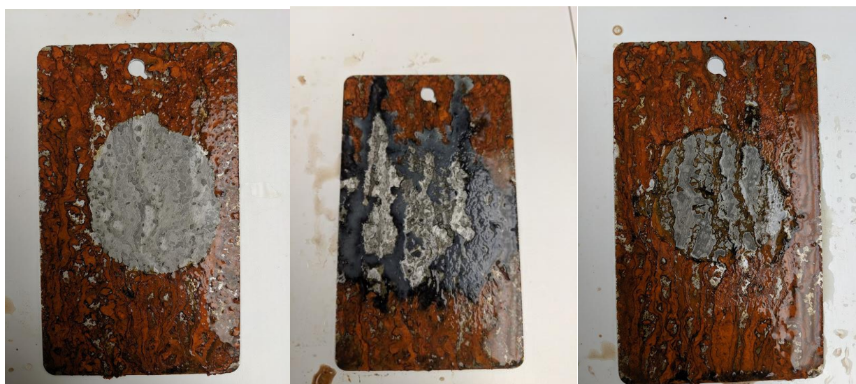
Figure 1: Panels after 1 hour of exposure to various rust removers. From left to right, VpCI-423, Evapo-Rust Gel, Nox-Rust Premium Rust Remover
