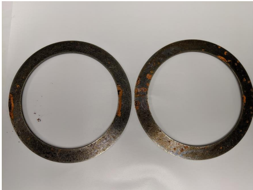
Figure 2: Rings from control group at 120 hours. Obvious signs of corrosion along the top surface, with small dark spots of corrosion seen as well.
