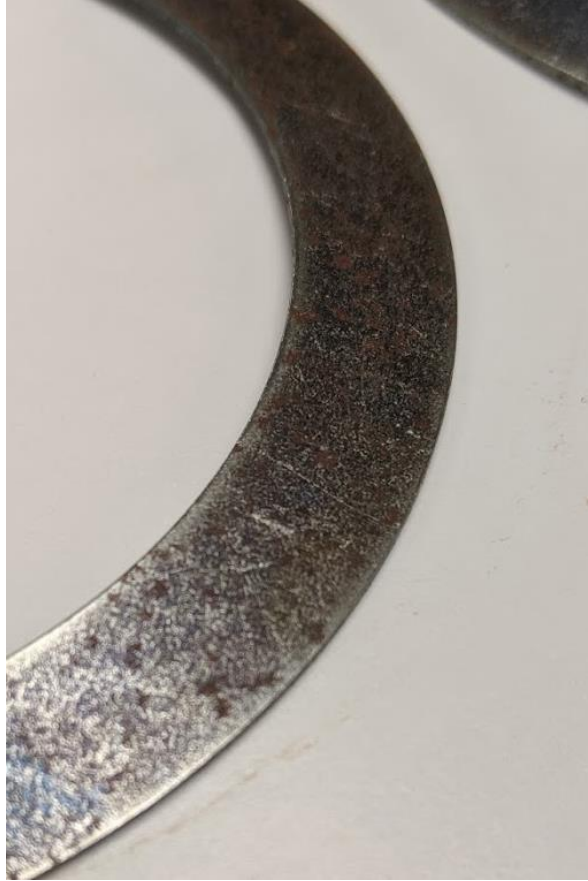
Figure 5: Close-up of a ring protected by yellow VCI film and silica desiccant. Small dark spots of corrosion can be observed on the surface.
