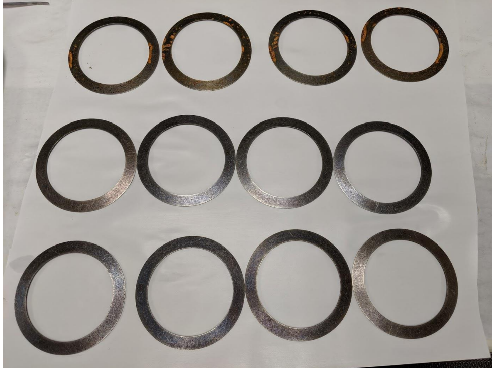
Figure 1: All rings after 120 hours of testing. The top row of rings is the control group. Middle row, VpCI-126 and DesiCorr protected. Bottom row, yellow VCI film and silica desiccant protected.
