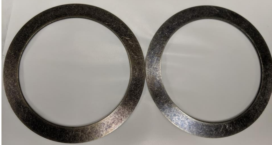
Figure 3: Close up of parts protected by VpCI-126 and DesiCorr. No signs of corrosion.
