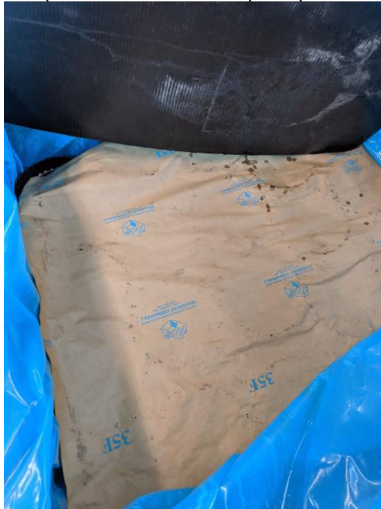
Figure 4: Top layer of paper, parts protected by VpCI-126 film. No significant water ingress occurred.
