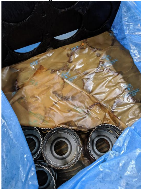
Figure 1: Parts protected by competitor VCI film. Heavy water ingress caused corrosion on the parts.
