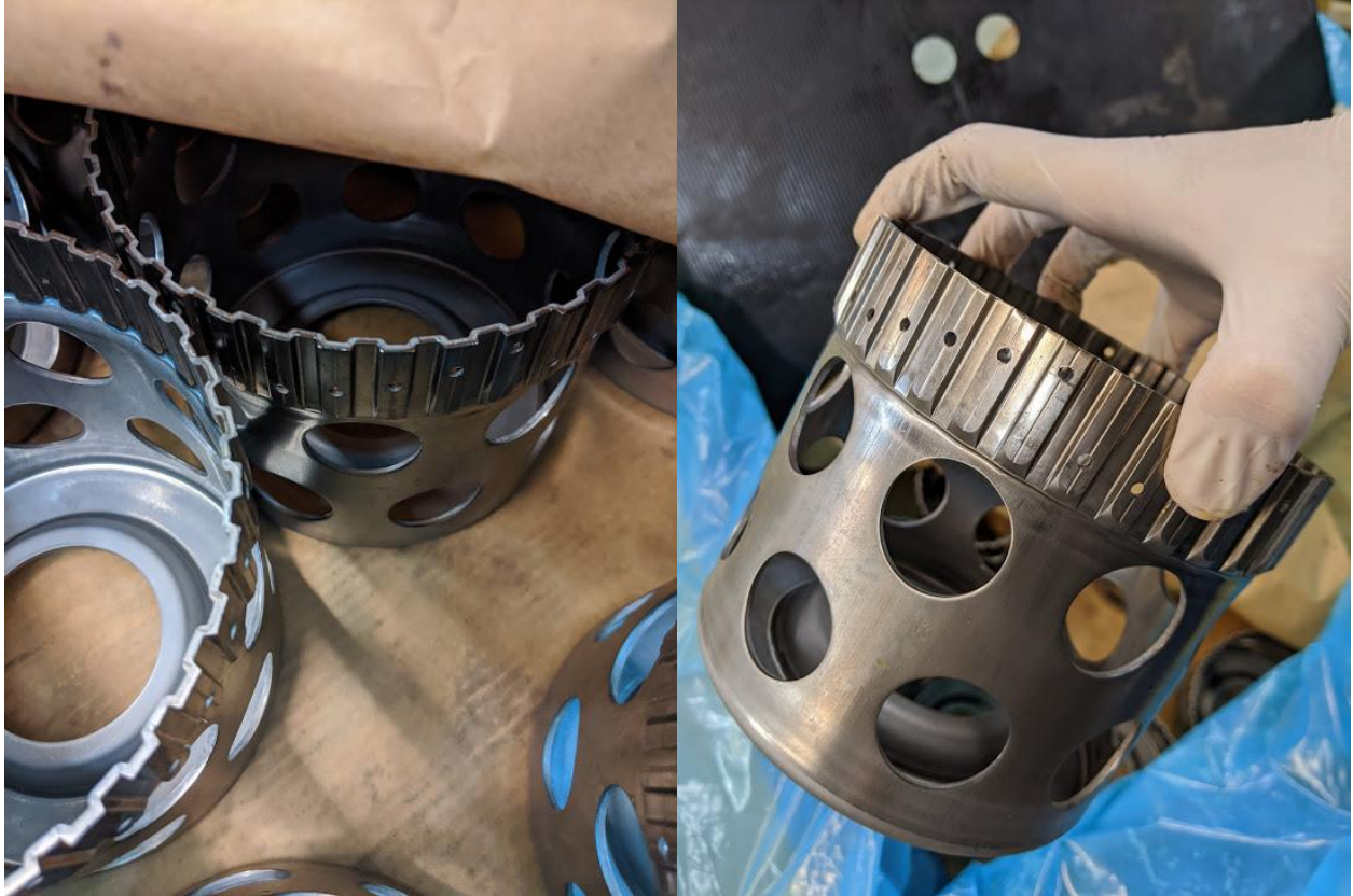
Figures 5 & 6: Parts protected by VpCI-126 film. No visible corrosion was seen on the parts.
