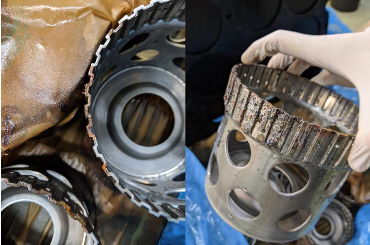
Figures 2 & 3: Close up view of corrosion on parts protected by competitor film.
