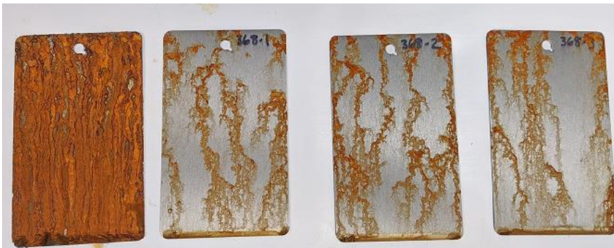
Figure 3: Panels treated by VpCI-368, diluted to match Anticorit SV-7X, in ASTM B-117 at 30.5 hours. Untreated panel on the left.
