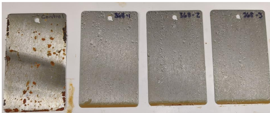
Figure 1: Panels protected by VpCI-368, diluted to match Anticorit SV-7X, in ASTM D-1735 at 120.5 hours. Untreated panel on the left.
