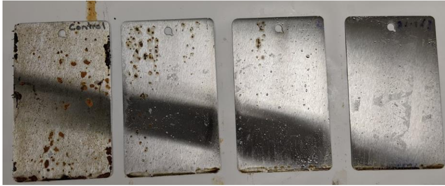
Figure 2: Panels protected by Anticorit SV-7X, in ASTM D-1735 at 120.5 hours. Untreated panel on the left. 2/3 panels showed signs of corrosion
