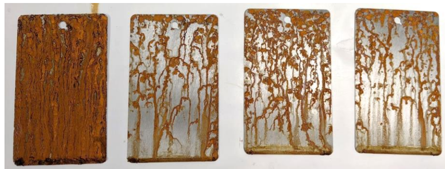
Figure 4: Panels treated with Anticorit SV-7X in ASTM B-117 at 30.5 hours. Untreated panel on the left.
