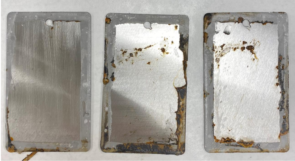
Figure 1: CT 1257 panels after 336 hours in humidity.
