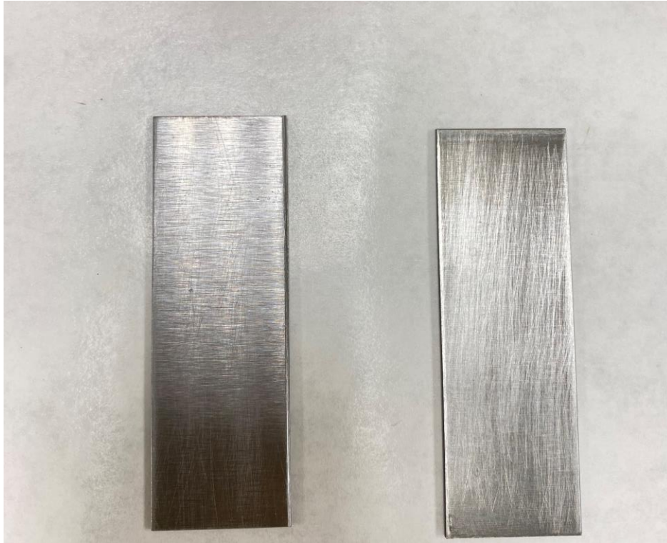
Figure 3: Panels (CT1257 left, VPCI-649 BD right) after 360 hours of half immersion testing. No corrosion on either panel.
