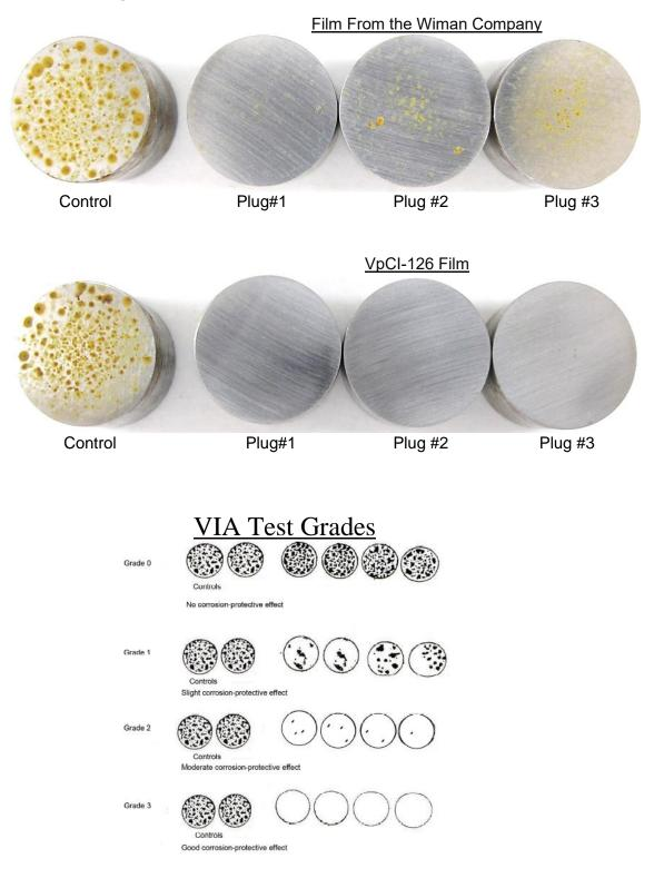
Interpretations: The film from the Wiman Company provides sufficient contact corrosion protection to pass the razor blade test for steel and copper. However, according to the results of the NACE VIA test, the Wiman film only provides a slight corrosion protective effect in the vapor phase. Cortec's VpCI-126 film provides a good corrosion protective effect in the vapor phase and also passes the razor blade test for steel and copper.
