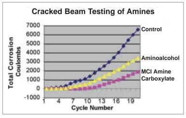
are attracted to both anodes and cathodes, which is how they can help reduce the amount of corrosion. MCI 2020 is a blend of organic inhibitors. Some of this blend has molecules with similar partial + and partial - charges. But, a majority of this blend consists of an amine carboxylate that reacts with the concrete as it migrates through.
