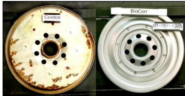
The study includes comparative experimental investigation of biobased and petroleum based rust preventives in humidity chamber, with the corrosion protection efficiency being determined using various polarisation techniques.
