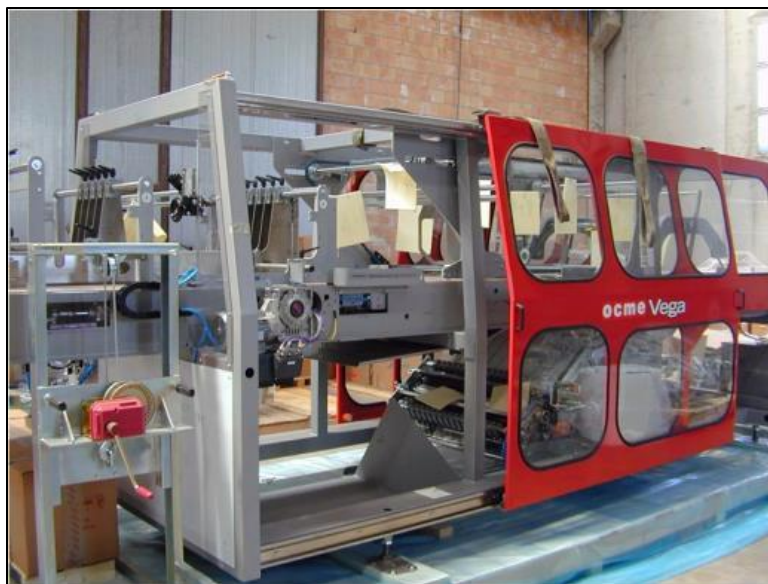
In transport corrosion protection using Cortec's VpCl® 132 foam for shrink wrapping machine for PET bottles.
