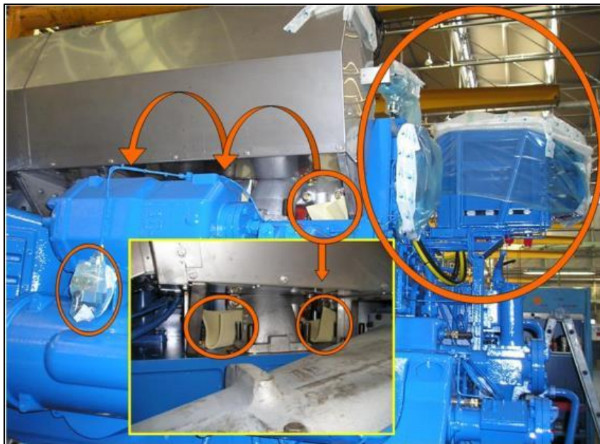
Ship's engine in Trieste, Italy, protected with VpCl foam (as marked in the picture) getting ready for ocean transport.
