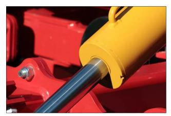
A more cost-effective and successful option is incorporating Vapor phase Corrosion Inhibitors (VpCIs) into hydraulic fluids where void space protection is needed. These corrosion inhibitors protect both the metal in contact with the fluid and metal surfaces above the fluid. When used, the amount of hydraulic fluid needed during storage or shipment can often be reduced at the same time protection is
