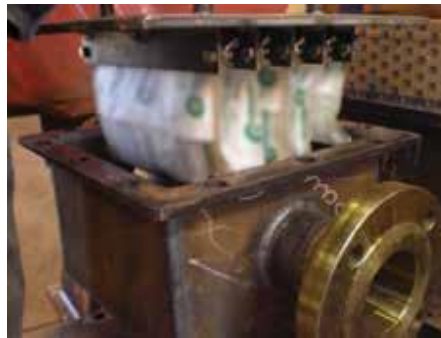
FIGURE 7 An example of a plenum that could be installed to introduce VCI A to a sprinkler system.
