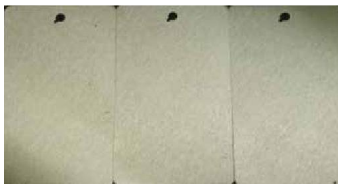
FIGURE 4 Panels treated with an inhibitor.
