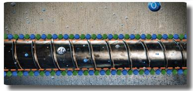
Migrating corrosion inhibitors work their way through concrete pore structures to form a protective molecular layer on embedded steel reinforcement. Image Credit:
