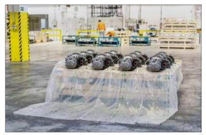
Cortec's VpCI®-126 Film and Bags are some of the most basic and versatile materials for automotive shipping and storage protection. Featuring the world's top-quality VpCI® Film Technology, VpCI®-126 packaging material forms a protective molecular layer on intricate and hard-to-reach metal surfaces inside the package. For the utmost convenience, parts can be used immediately after coming out
